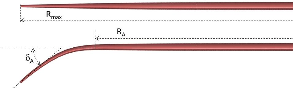
Figure 3. Explanation of design parameters influencing the blade-tip anhedral.
