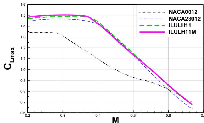
Figure 5. The dependency: maximum lift coefficient ( $C_{Lmax}$ ) versus Mach number ( $M$ ) determined computationally for the airfoils: ILULH11, ILULH11M, NACA23012 and NACA0012.
