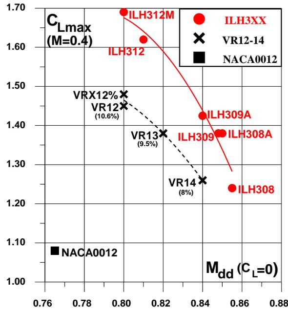
Figure 2. Computational aerodynamic characteristics of designed airfoil family ILH3XX and reference family VR12-14. Dependency  $C_{Lmax}$  at  $M=0.4$  versus  $M_{dd}$  at  $C_L=0$  [7].
