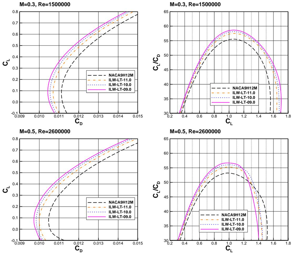
Figure 7. Comparison of aerodynamic characteristics of gyroplane airfoils ILW-LT-09.0, ILW-LT-10.0, ILW-LT-11.0 and NACA 9H12M, for flight conditions  $M=0.3, Re=1500000$  and  $M=0.5, Re=2600000$ .
