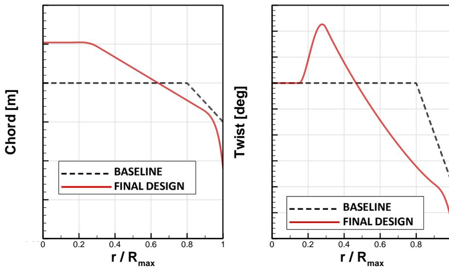
Figure 4. Comparison of radial distributions of blade chord (left graph) and geometrical twist (right graph), for the BASELINE blade and eventually designed blade (FINAL DESIGN).
