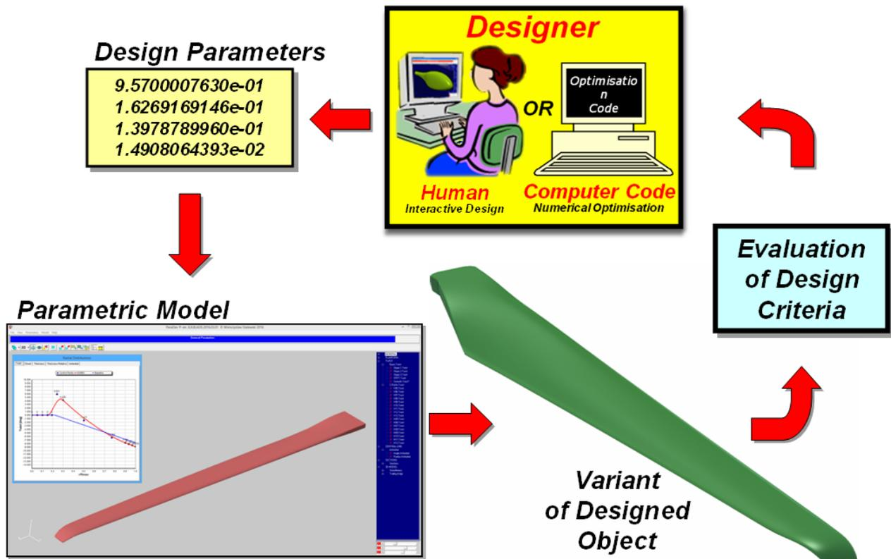
Figure 1. The general scheme of the developed and applied methodology of parametric design and optimisation of rotorcraft rotors.
