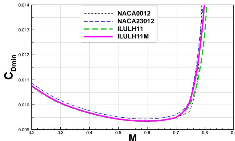
Figure 6. The dependency: minimum drag coefficient ( $C_{Dmin}$ ) versus Mach number ( $M$ ) determined computationally for the airfoils: ILULH11, ILULH11M, NACA23012 and NACA0012.
