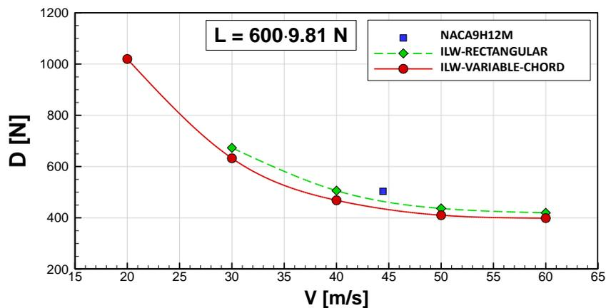
Figure 9. Total drag force ( $D$ ) acting on the rotor versus flight velocity ( $V$ ), during the flight of the gyroplane of total mass 600 kg. Comparison of computational results for reference rotor NACA9H12M and for newly designed and optimised rotors ILW-RECTANGULAR and ILW-VARIABLE-CHORD.
