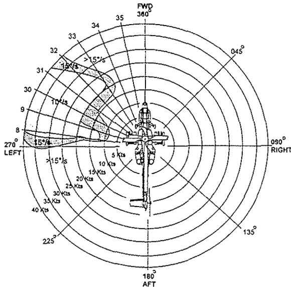
**Figure 8: Vertical Stabilizer Configuration 3: Out-of-wind Hover Envelope and Yaw Rate**
