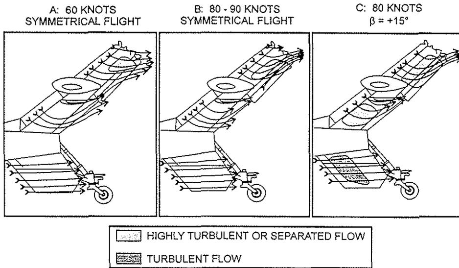
In an attempt to gain a better understanding of the flow mechanisms involved on the dorsal and ventral fins, the surface flow on the post side (curved side) of the dorsal and ventral stabilizers were investigated by using wool tufts stuck to the surface of the stabilizers. The results are shown in figure 4.
