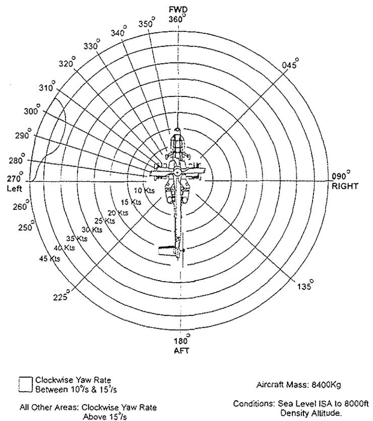
Figure 10: Vertical Stabilizer Configuration 4: Out-of-wind Hover Envelope and Yaw Rate Envelope
