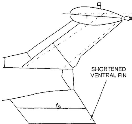
Figure 9: Vertical Stabilizer Configuration 4: Geometry
