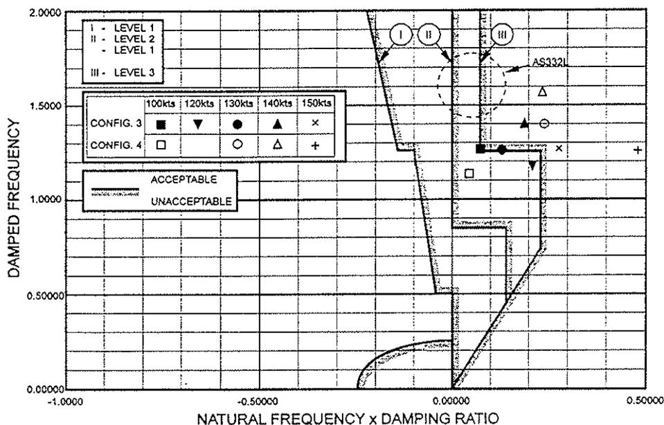
**Figure 11: Vertical Stabilizer Configuration 4: Lateral-Directional Dynamics Stability Characteristics**
