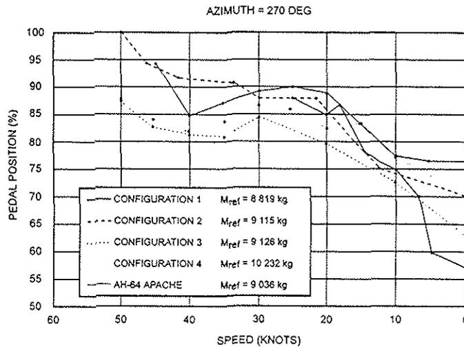
Figure 2: Yaw Pedal Position vs. Sideways Speed 270° Azimuth
