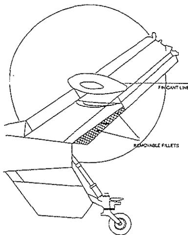
Figure 1: Vertical Stabilizer Configuration 1: Geometry
