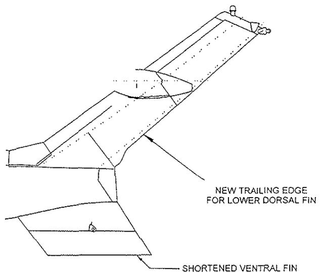
**Figure 7: Vertical Stabilizer Configuration 3: Geometry**
