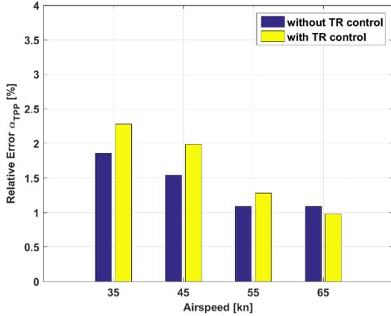
Figure 5: Percent observation error on  $\alpha_{\text{TPP}}$  for changing airspeed. Check on airspeeds not used for identification.
