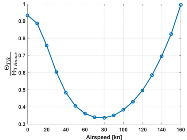
Figure 4: Normalized value of  $\theta_{TR}$  for trim as a function of the airspeed.
