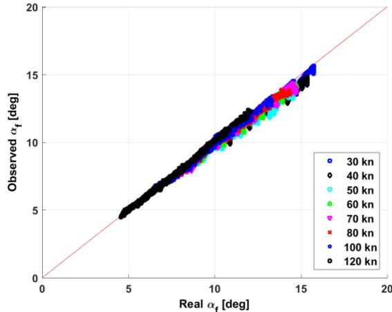
Figure 12: Observation quality test on  $\alpha_{fus}$  at several airspeeds.
