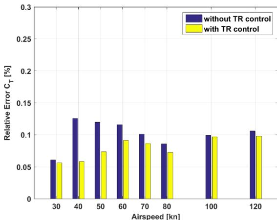
Figure 2: Percent observation error on the samples used for identification, as a function of the airspeed. Comparison between augmented and standard model. Top plot:  $\alpha_{TPP}$ . Bottom plot:  $C_T$ .
