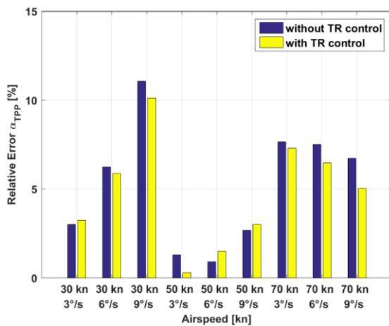
Figure 8: Percent observation error on  $\alpha_{TPP}$  in off-design coordinated turns, for changing airspeed and turn rate. Comparison between augmented and standard model.
