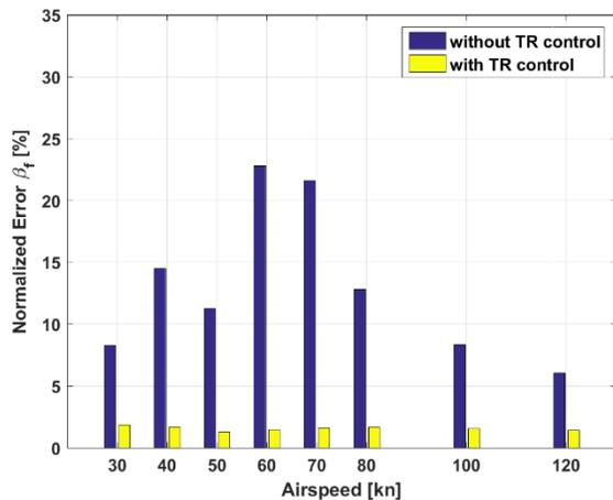
Figure 10: Percent observation error on  $\beta$  for changing airspeed. Comparison between augmented and standard model. Samples not used for identification.
