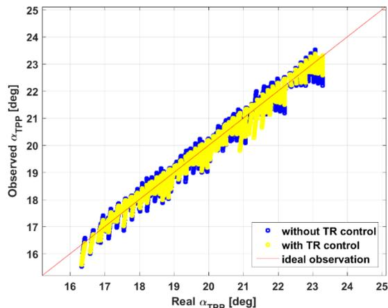
Figure 1: Observation quality test on  $\alpha_{TPP}$  at  $V = 50$  kn. Comparison between augmented and standard model.
