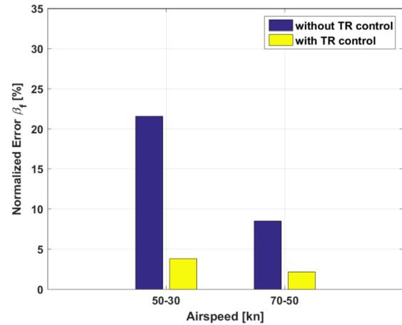
Figure 11: Percent observation error on  $\beta$  in off-design decelerated descents, as a function of the airspeed. Comparison between augmented and standard model.
