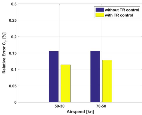
Figure 7: Percent observation error in off-design decelerated descents, as a function of the airspeed. Comparison between augmented and standard model. Top plot:  $\alpha_{TPP}$ . Bottom plot:  $C_T$ .
