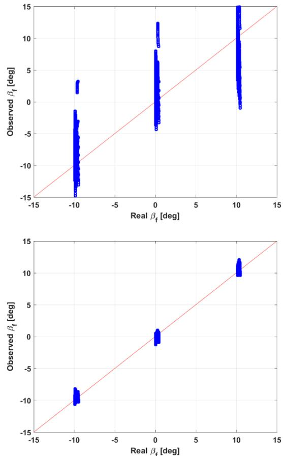
Figure 9: Observation quality test on  $\beta$  at  $V = 50$  kn. Comparison between standard (top plot) and augmented model (bottom plot).
