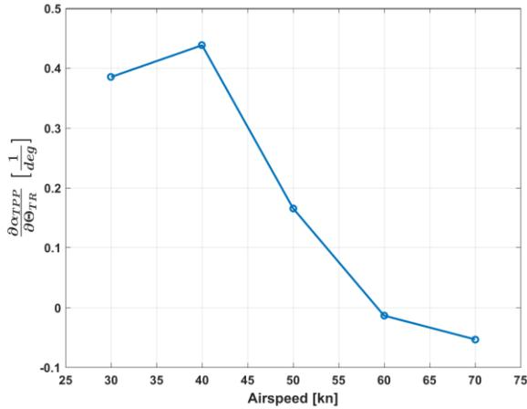
Figure 6: Dependence of the model coefficient  $\frac{\partial \alpha_{\text{TPP}}}{\partial \theta_{\text{TR}}}$  on the airspeed.
