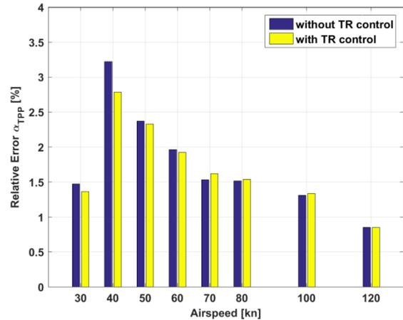
Figure 3: Percent observation error on  $\alpha_{TPP}$  for changing airspeed. Check on sideslip values not used for identification.
