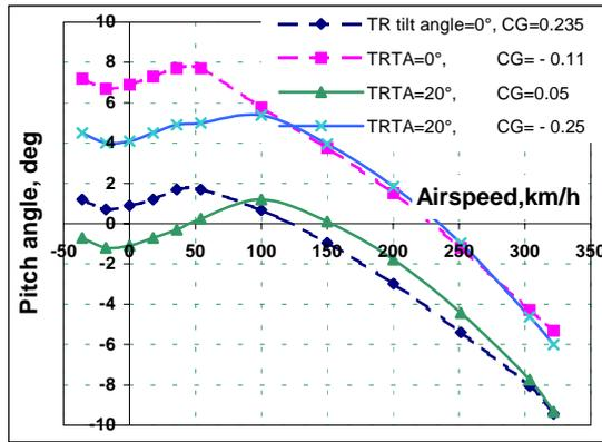
**Fig. 23. MI-24 pitch angle vs. airspeed**
