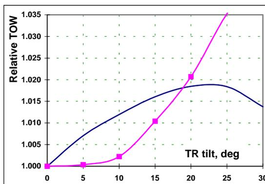
**Fig. 8. Increase in MI-24 total lift due to both TR tilt and increase in power transmitted to MR**
