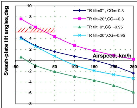
Fig. 12. Swash-plate angles need for level flight
