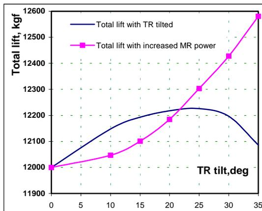
**Fig. 7. Increase in MI-8 total lift due to both TR tilt and increase in power transmitted to MR**
