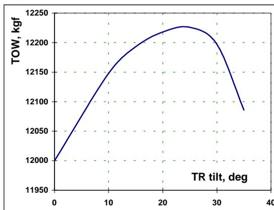
**Fig. 3. MI - 8 total lift vs. TR tilt angle**
