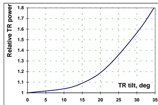
**Fig. 6. MI-24 TR power required for hover ceiling vs. TR tilt angle**
