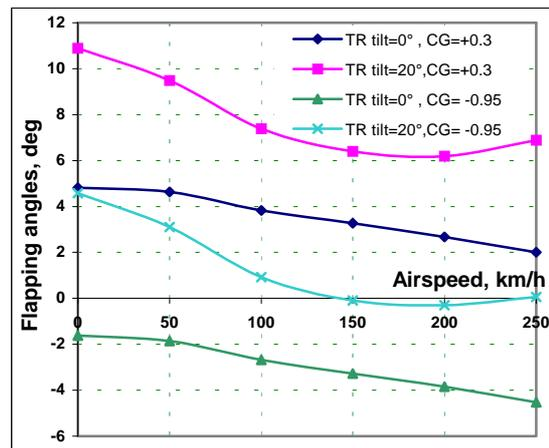
Fig. 15. MR blades flapping angles at 180° azimuths vs. airspeed.
