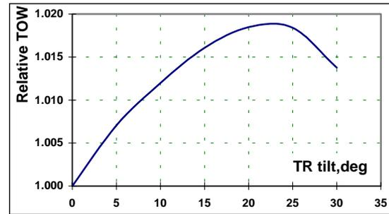
**Fig. 4. MI-24 relative total lift vs. TR tilt angle**
