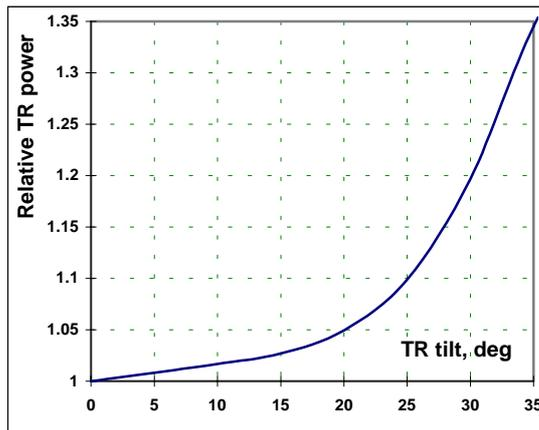
**Fig. 11. Impact of TR tilt of a new light helicopter on TR power required**
