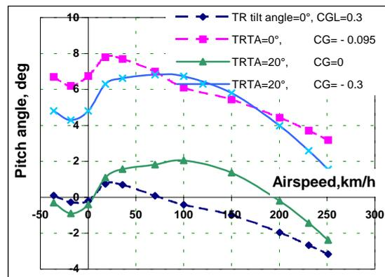
Fig. 22. MI-8 pitch angle vs. airspeed
