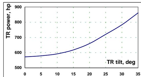
**Fig. 5. MI -8 TR power required for hover ceiling vs. TR tilt angle**
