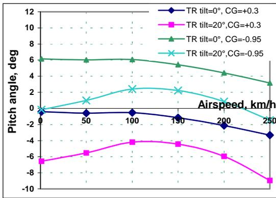
Fig. 13. Pitch angles of MI-8 helicopter
