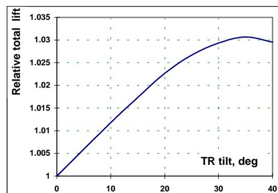
**Fig. 10. New helicopter total lift vs. TR tilt**
