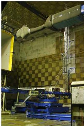
Figure 1: HART hingeless model rotor in the DNW wind tunnel.
