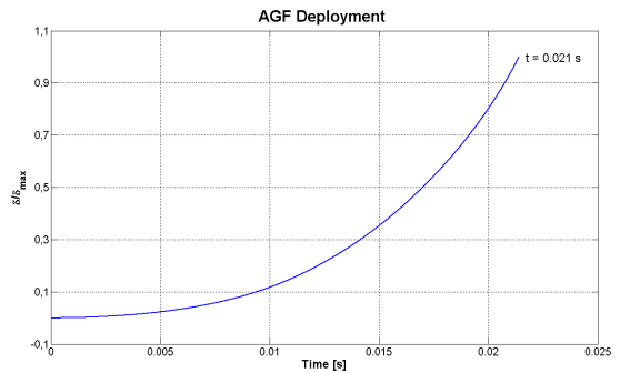
Figure 12: Numerical estimation of AGF deployment time
