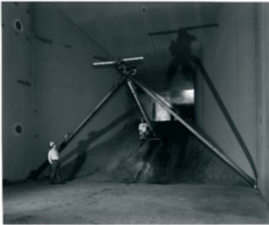
Figure 3: Facility used to conduct interference-free axial flow experiment 48 for a 2-bladed rotor in the Ames 30x30 settling chamber of the 7 x 10 tunnel.
