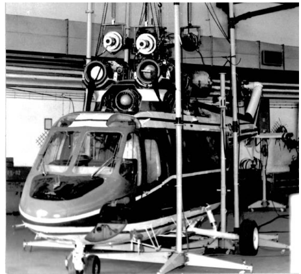
Figure 5. General layout of the PZL W-3A helicopter modal tests.
