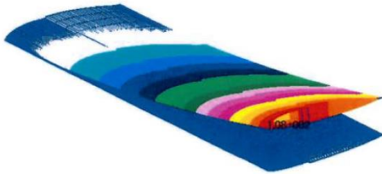
Figure 2. FEM model of the new MR blade mid part.
