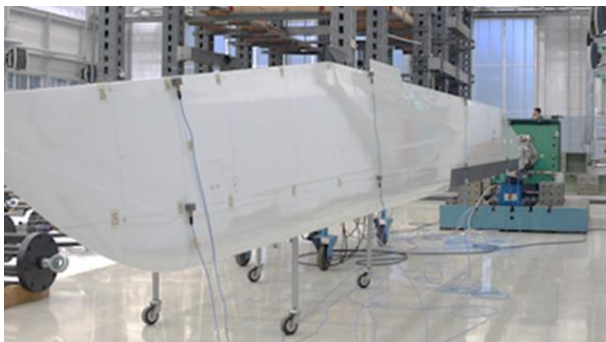
Figure 13. General layout of the ground modal test of the new W-3A helicopter MR blades.
