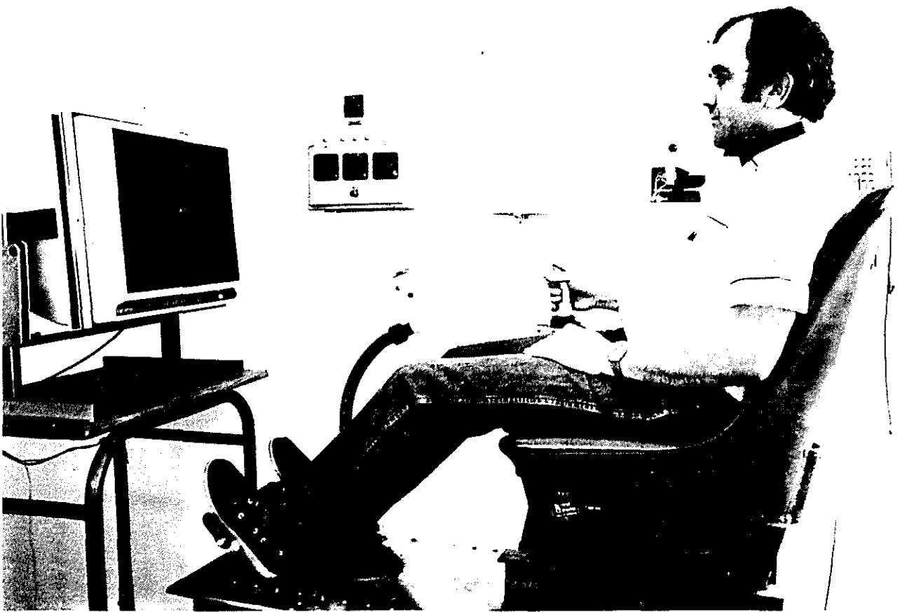
Fig. 1 - Experimental setup showing the vibrating platform supporting the seated subject. The spot target was presented on the screen of the oscilloscope. The tracking target was actuated by either the conventional stick or the mini-stick (placed on the right hand side of the subject), both equipped with potentiometric and strain gauge devices for position and force controls, respectively.
