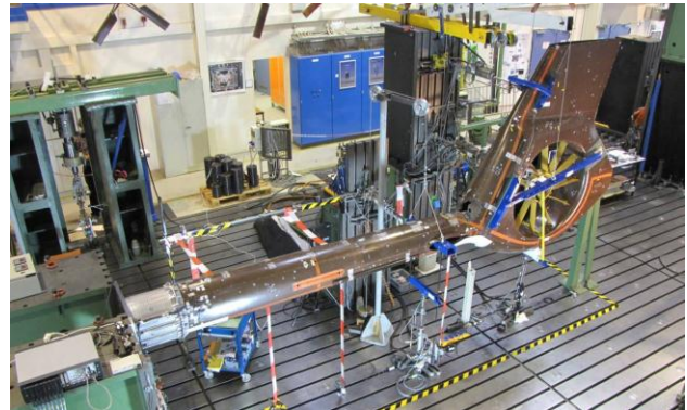
Fig.17: Test set up for a composite tail boom full scale test.
