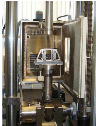
Fig.14: Test setup for \sigma_{CAI} static & fatigue testing
