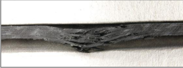
Fig.3: Typ. delamination of a monolithic part after an impact with 9J.
