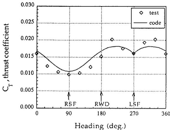
Fig. 14 OH-58 tail rotor thrust coefficient variation with heading (45 kts, collective = 19°)
