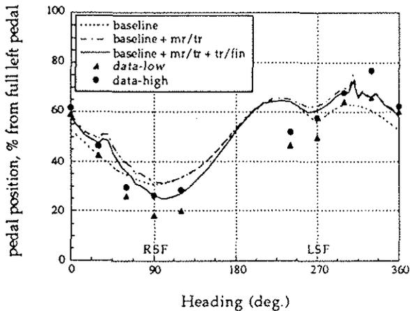
Fig. 24 SH-2 critical azimuth results compared with flight test data (speed = 35 knots)
