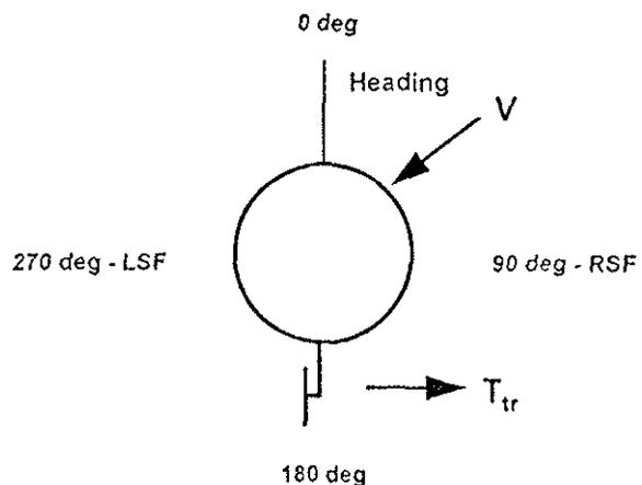
Fig. 1 Top view of single main rotor helicopter in yawed flight
