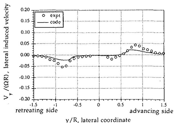
Fig. 7 Comparison of lateral velocities induced at  $0.29R$  below the main rotor hub
