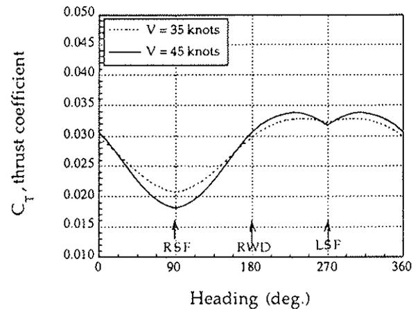
Fig. 16 SH-2 thrust coefficient variation with heading (collective = 19°)
