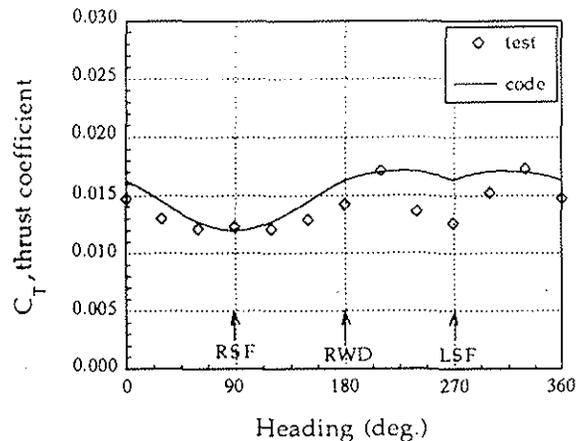
Fig. 13 OH-58 tail rotor thrust coefficient variation with heading (35 kts, collective = 19°)
