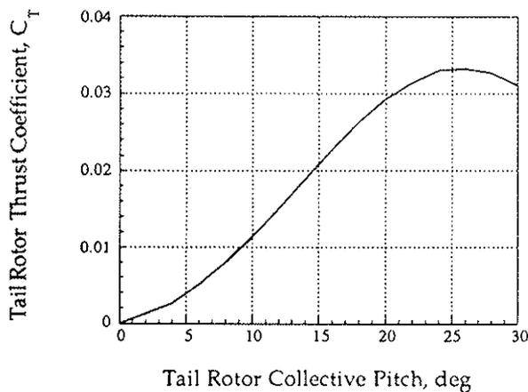
Fig. 15 Calculated isolated SH-2 tail rotor thrust coefficient in hover
