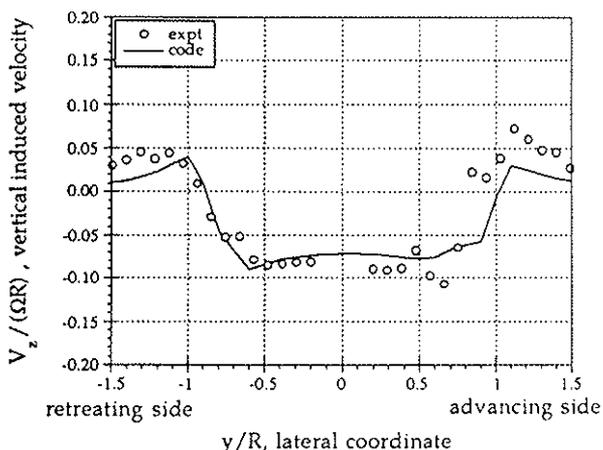
Fig. 10 Vertical induced velocity 1.05R behind the main rotor
