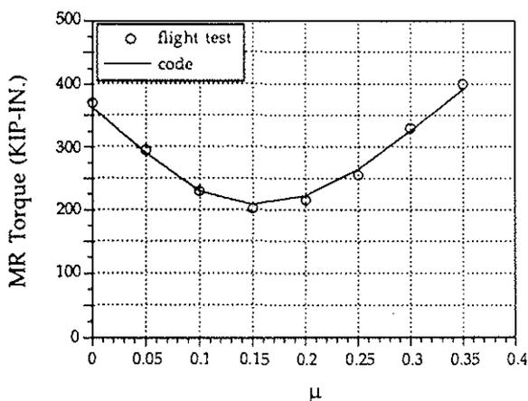
Fig. 2 SH-2 Main Rotor Torque ( $C_T/\sigma = 0.0725$ )
