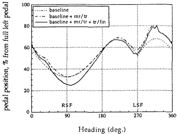
Fig. 25 SH-2 critical azimuth results (speed = 45 knots) - no flight test data available
