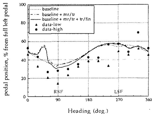
Fig. 22 SH-2 critical azimuth results compared with flight test data (speed = 25 knots)
