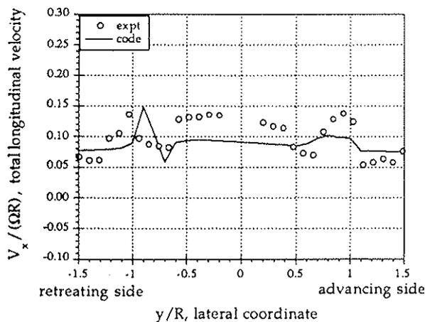
Fig. 8 Total longitudinal velocity 1.05R behind the main rotor (free stream plus induced velocity)
