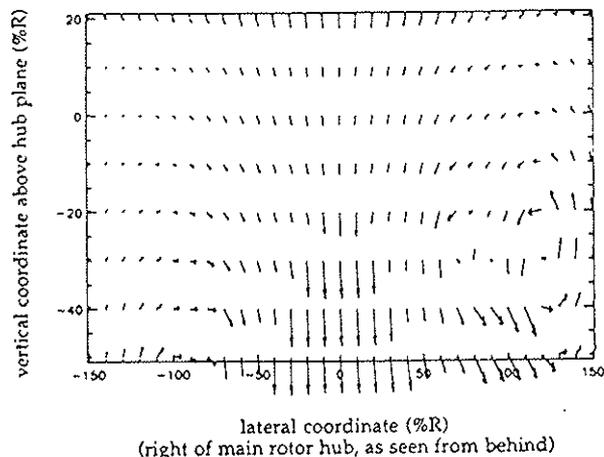
Fig. 27 Velocity vector plot 1.2045R behind the SH-2 main rotor hub (speed = 35 knots,  $\mu = 0.086$ )
