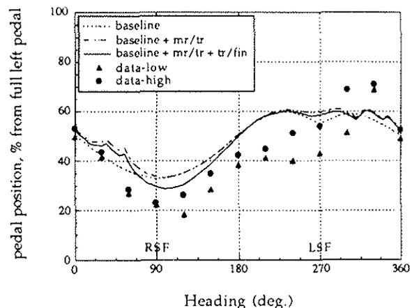
Fig. 23 SH-2 critical azimuth results compared with flight test data (speed = 30 knots)
