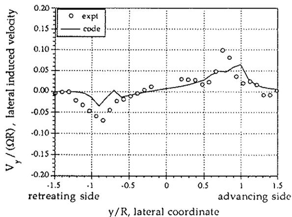
Fig. 9 Lateral induced velocity 1.05R behind the main rotor
