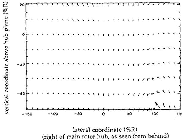
Fig. 26 Velocity vector plot 1.2045R behind the SH-2 main rotor hub (speed = 20 knots,  $\mu = 0.05$ )
