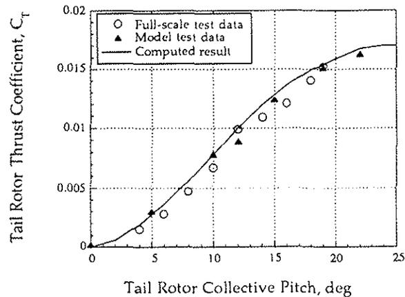
Fig. 12 Comparison of predicted OH-58 isolated tail rotor thrust coefficient in hover with test data
