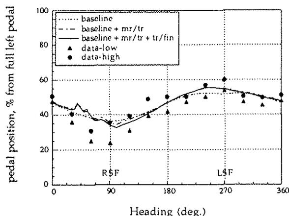
Fig. 21 SH-2 critical azimuth results compared with flight test data (speed = 20 knots)
