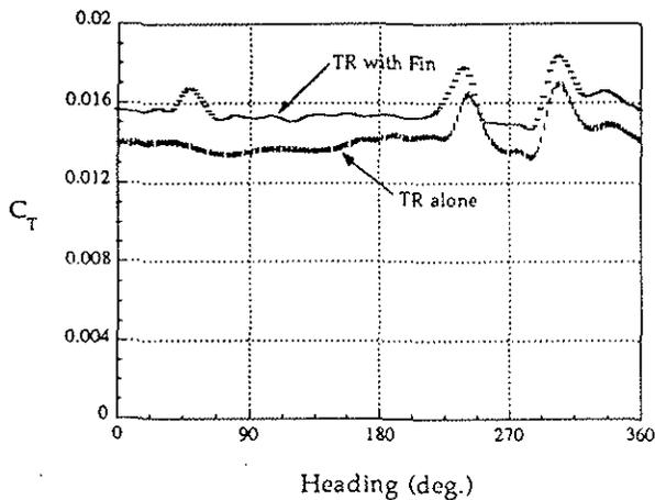
Fig. 17 Effect of Fin on OH-58 Tail Rotor Thrust Coefficient [7], collective = 19°, V = 20 knots
