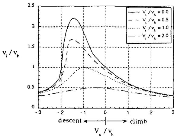
Fig. 11 Variation of induced velocity with climb and forward flight velocity
