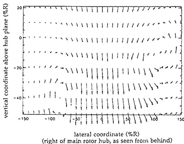
Fig. 28 Velocity vector plot 1.2045R behind the SH-2 main rotor hub (speed = 45 knots,  $\mu = 0.11$ )
