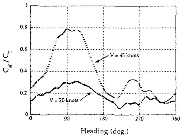
Fig. 18 Variation of OH-58 Empennage Side Force Coefficient as a ratio of tail rotor thrust coefficient, collective = 19°, blockage ratio = 0.44
