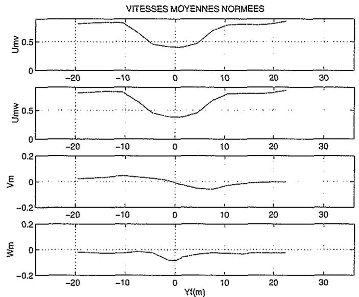
Figure 6 : Mean velocities evolution along the lateral axis on the deck centre (pt A, height=4.4m) - Wind = 50 kts,  $\beta = 0^\circ$
