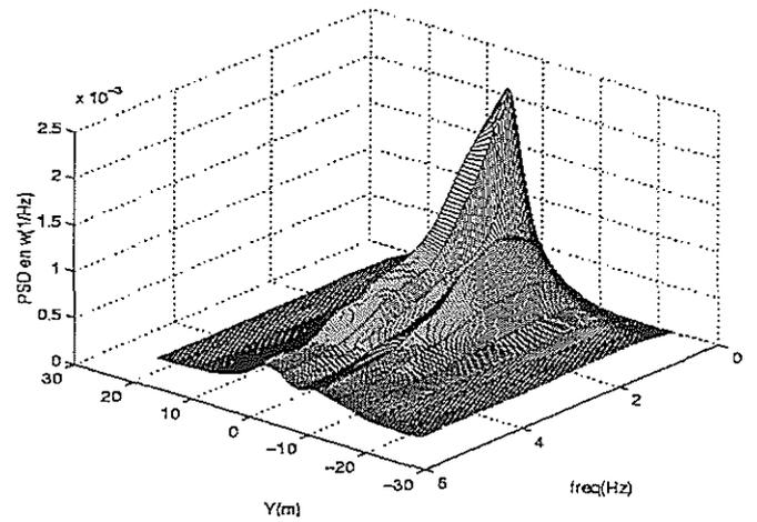
Evolution along the lateral axis on the deck centre (height 2.4m)
