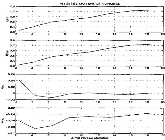
Figure 5 : Mean velocities evolution along the vertical axis on the deck centre (pt A) - Wind = 50 kts,  $\beta = 0^\circ$
