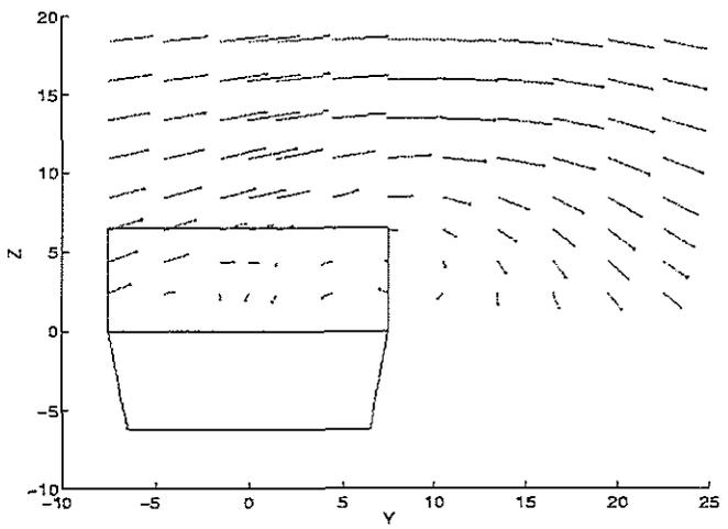
Figure 11 : Lateral section of the flow on plane n° 8
