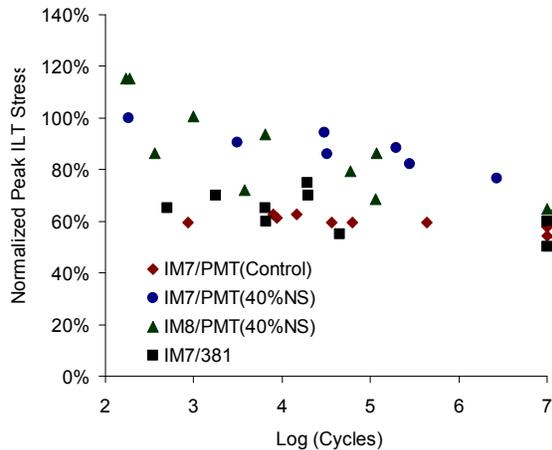
**Figure 15.** ILT fatigue data for 250° F curing carbon composites with and without nanosilica
