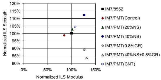
**Figure 9.** ILS strength and modulus results for 350° F curing carbon composites
