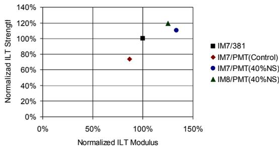
**Figure 14.** ILT strength and modulus results for 250° F curing carbon composites
