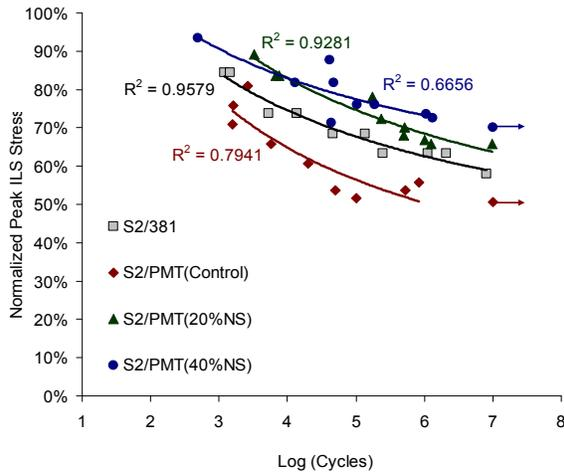
**Figure 8.** ILS S-N curves for 250° F curing S2-glass composites with and without nanosilica
