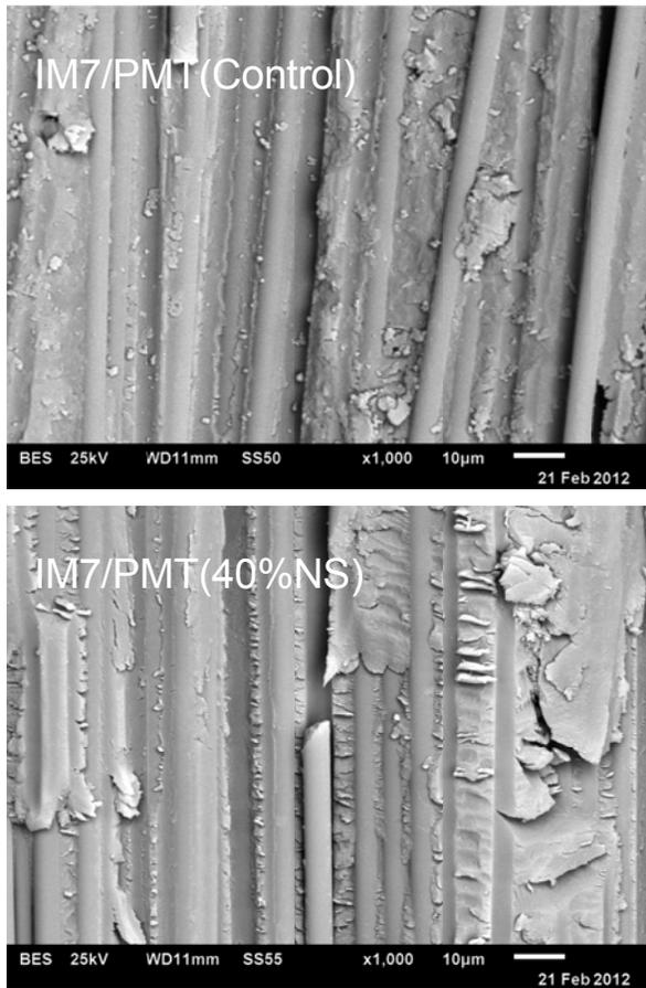
**Figure 11.** SEM images of ILS failure surfaces of 350° F curing carbon prepreg composites (1,000 x)
