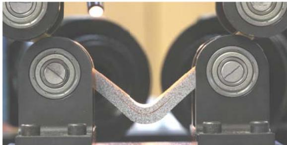
**Figure 13.** ASTM D 6415 test setup and tensile delamination failure of a unidirectional CB specimen
