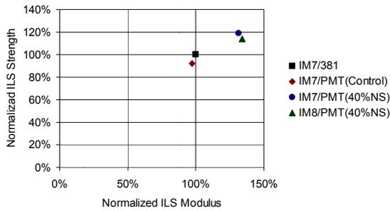
**Figure 5.** ILS strength and modulus results for 250° F curing carbon composites with and without nanosilica
