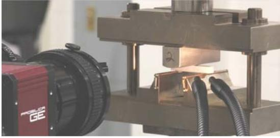
**Figure 4.** Modified SBS test setup for measuring ILS modulus, strength, and fatigue performance [10, 11]
