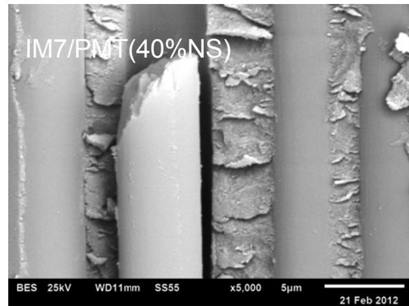
**Figure 12.** SEM images of ILS failure surfaces of 350° F curing carbon prepreg composites (5,000 x)
