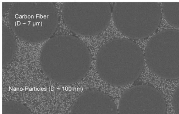
**Figure 1.** SEM image of a carbon/epoxy laminate cross section demonstrating even dispersion and lack of conglomeration for the nanosilica particles [4, 5]
