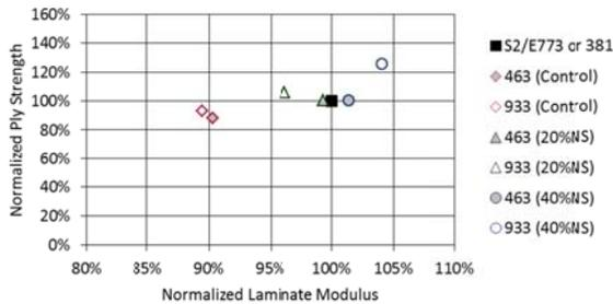
**Figure 3.** Compression results for 250° F curing S2-glass composites with and without nanosilica (notation for PMT prepregs starts with a number corresponding to AGY sizing)
