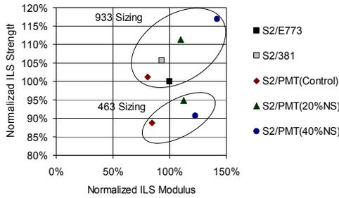
**Figure 7.** ILS strength and modulus results for 250° F curing S2-glass composites
