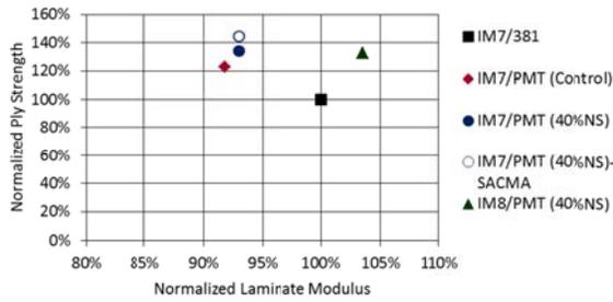
**Figure 2.** Compression results for 250° F curing carbon composites with and without 40% nanosilica
