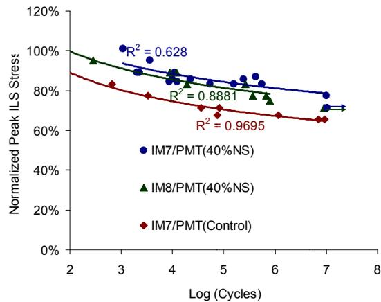
**Figure 6.** ILS S-N curves for 250° F curing carbon composites with and without nanosilica
