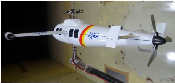
Figure 3 : Wind tunnel testing of a compound helicopter model in 2018 [14].
