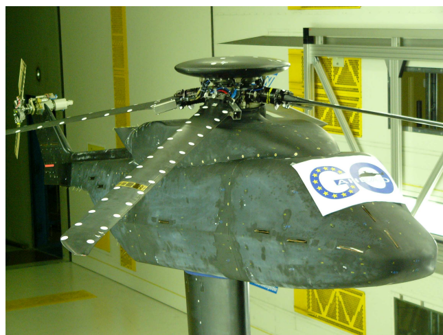
Fig. 1. GoAHEAD helicopter model in the DNW wind tunnel
