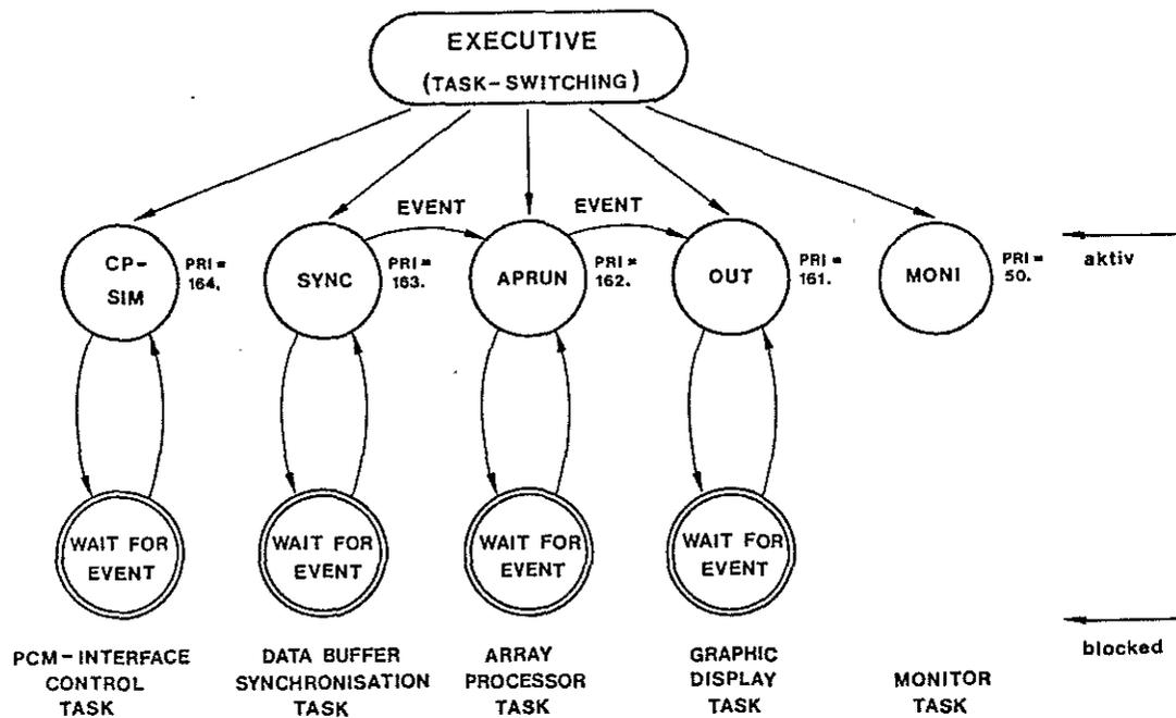
Figure 13. Software Configuration in the Quick-Look Processor System
