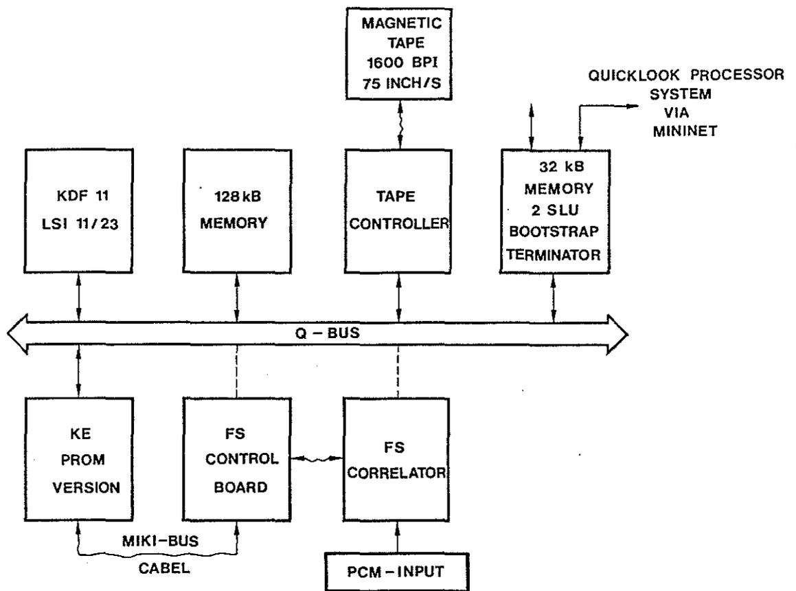
Figure 16. Data Acquisition and Supervise System Architecture
