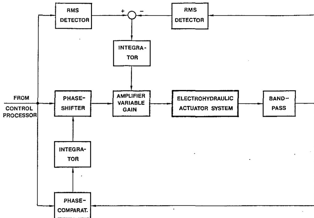
Figure 18. Closed Loop Control, Block Diagram
