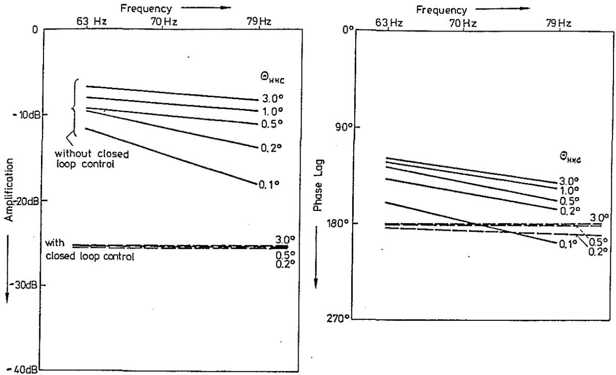
Figure 17. Frequency Response of an Actuator System, with and without Closed Loop Control
