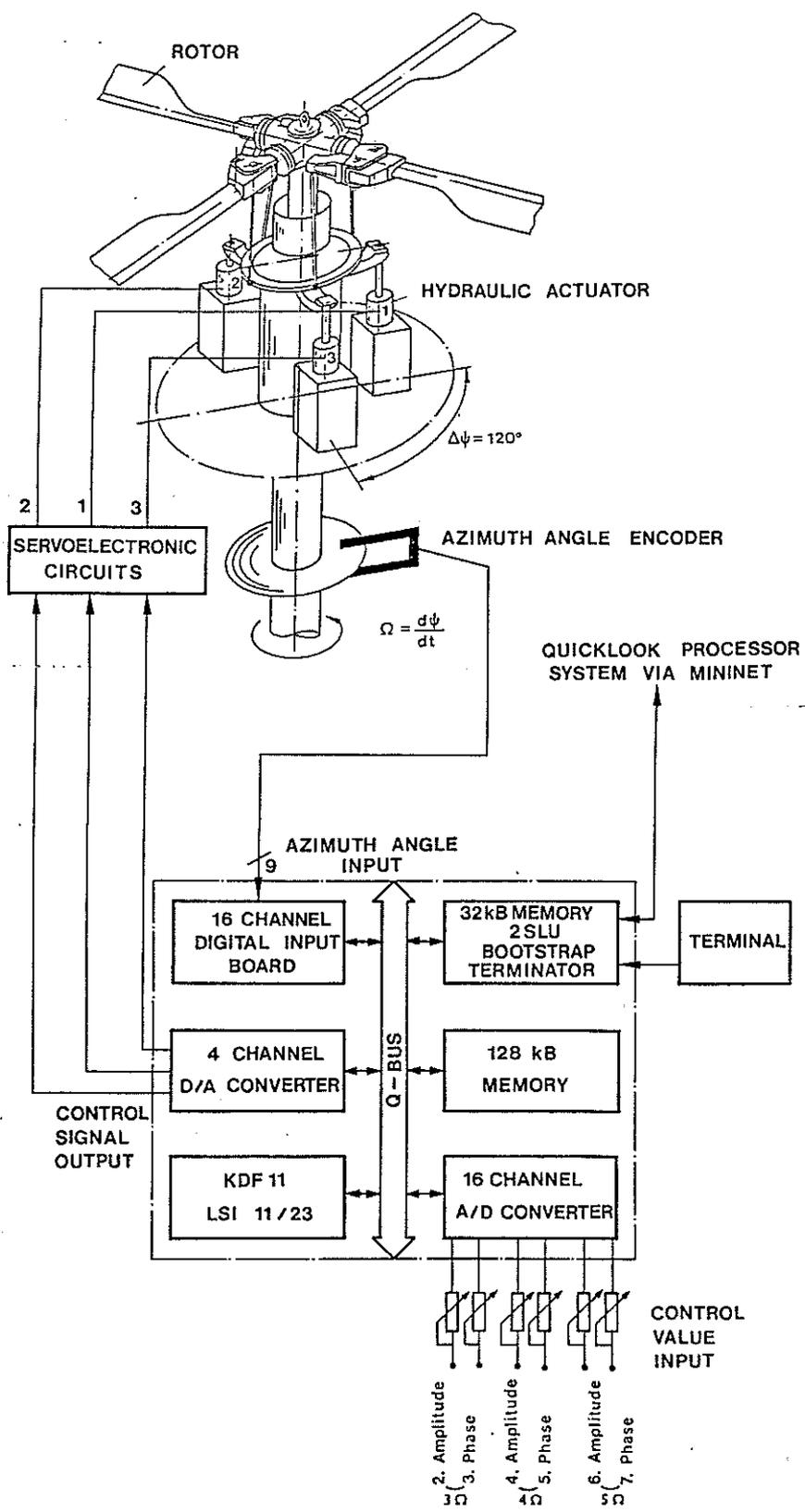
Figure 14. Control Processor Configuration
