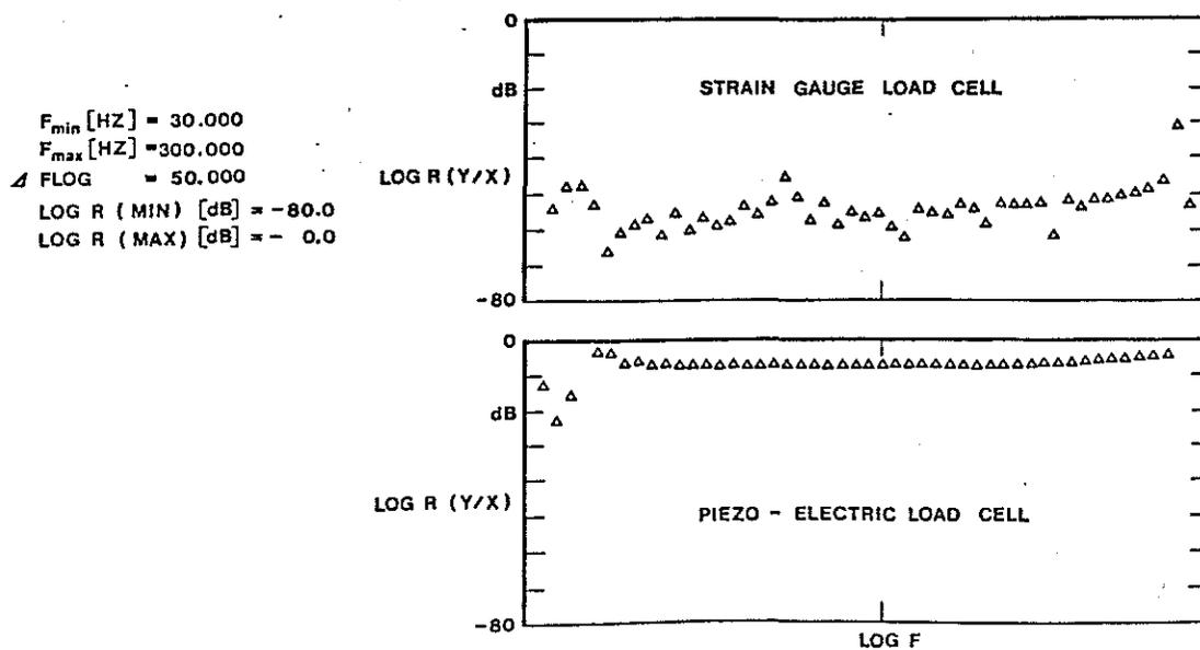
Figure 7. Frequency Response of the Force Transducers at 10 N Dynamic Loads
