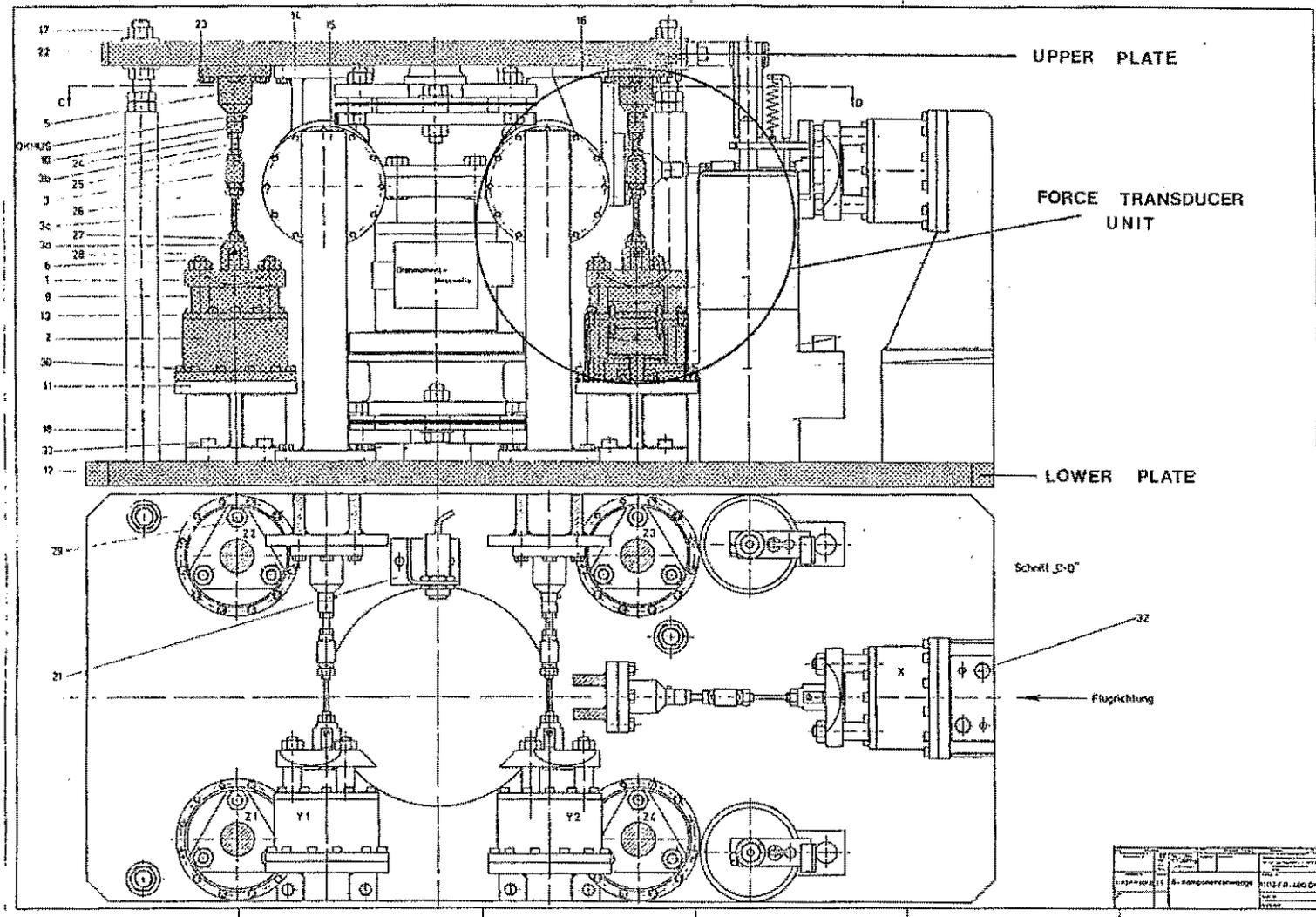
Figure 5. Six-Component Balance, Side View and Top View
