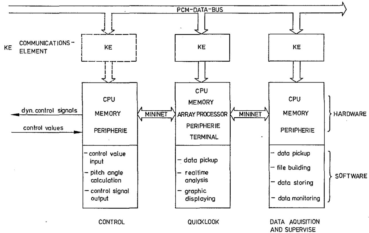
Figure 10. Digital Data Processing and Control System, Block Diagram
