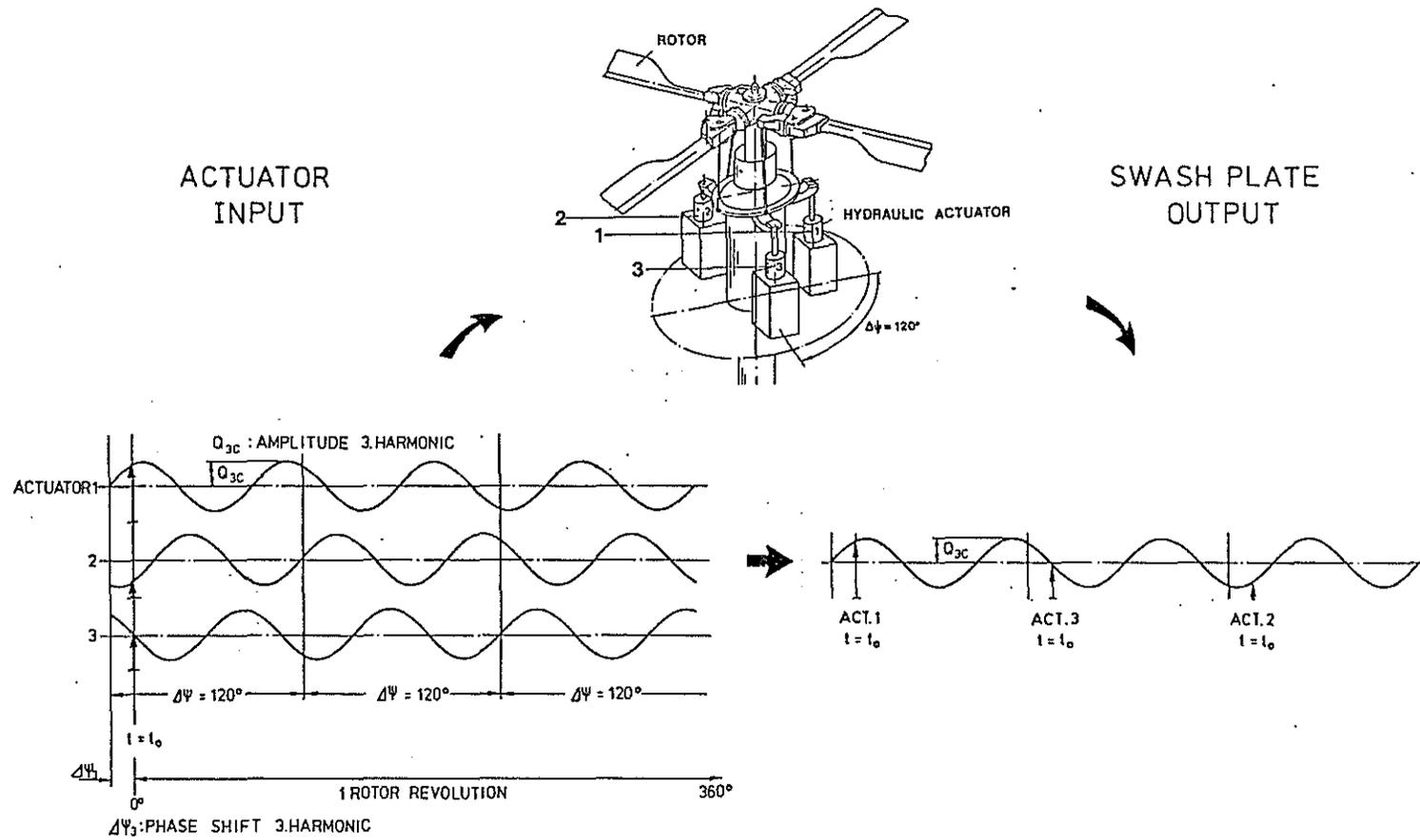
Figure 3. Interdependence of the Actuator Input and the Swash Plate Moving
