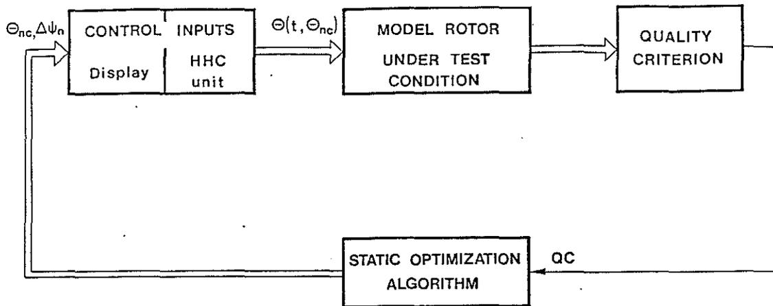
Figure 15. Principle of the Optimization Procedure
