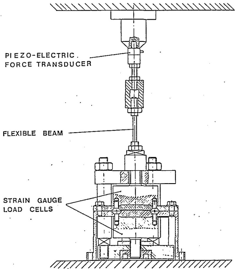
Figure 6. Force Transducer Assembly
