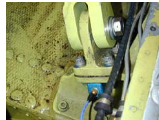
Figure 6. Detail view of the error sensor located on the strut connection support.
