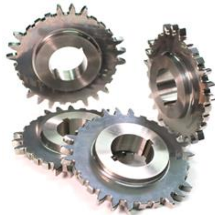
Figure 4. Fully processed STBF test gears built from Ferrium C64 steel powder, processed by DMLS deposition on an EOS M280, hot isostatic pressing, machining, carburization and heat treatment, final machining, shot peening and superfinishing.
