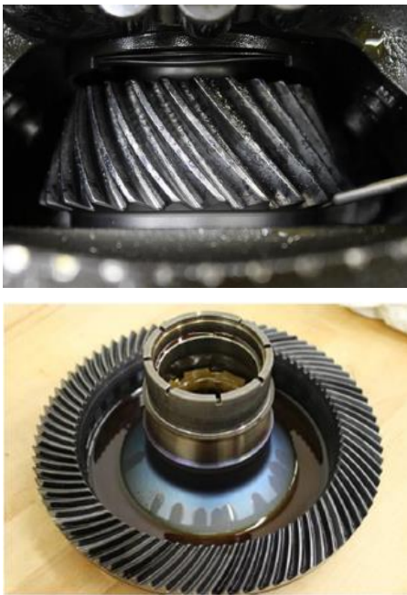
Figure 2. Ferrium C64 input shaft (top) and gearshaft (bottom) imaged after 85 minutes of loss-of-lubrication testing in the Bell FARDS program loss-of-lubrication testing, showing minor scuffing on the gear teeth but no signs of surface damage or failure. 3
