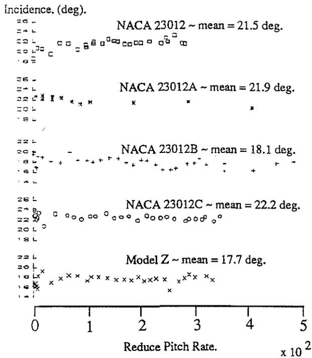
**Figure 6. Reattachment point variation with increasing pitch rates.**
