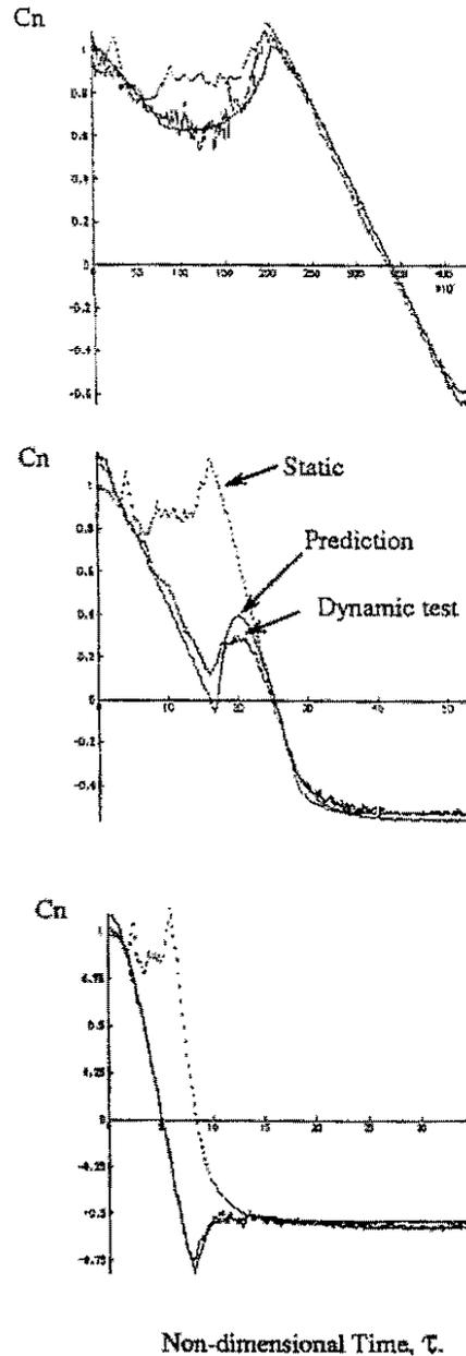
3. The presence of the wake takes a finite time to diminish, until which it remains a significant component in determining the airloads.
