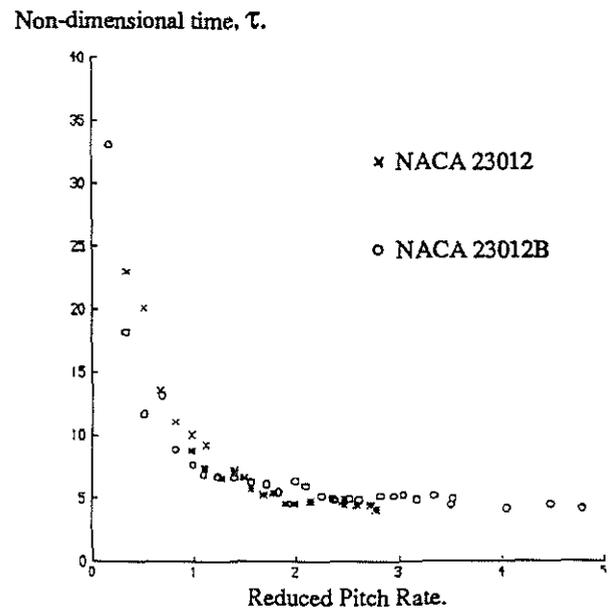
reattachment and downstream advancement can occur. Once the effect of aerofoil geometry has been suppressed, i.e., at high ramp-down pitch rates, the rate of reattachment is determined by the detailed fluid mechanics of this process.
