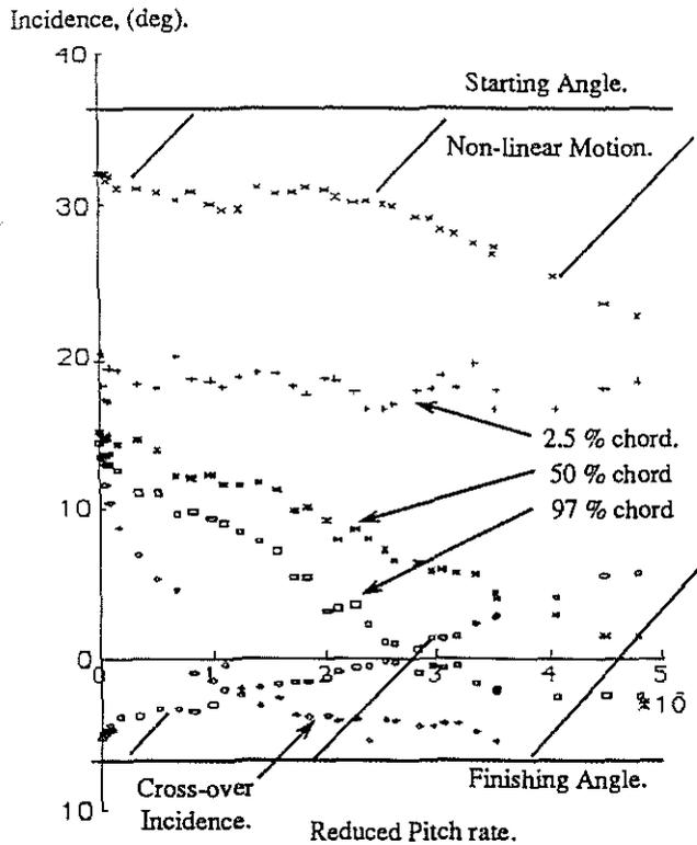
pitch rate above 0.015, the effect of aerofoil geometry is significantly reduced allowing the full reattachment time delay to approach a value of 4; equivalent to 25% of the freestream velocity.
