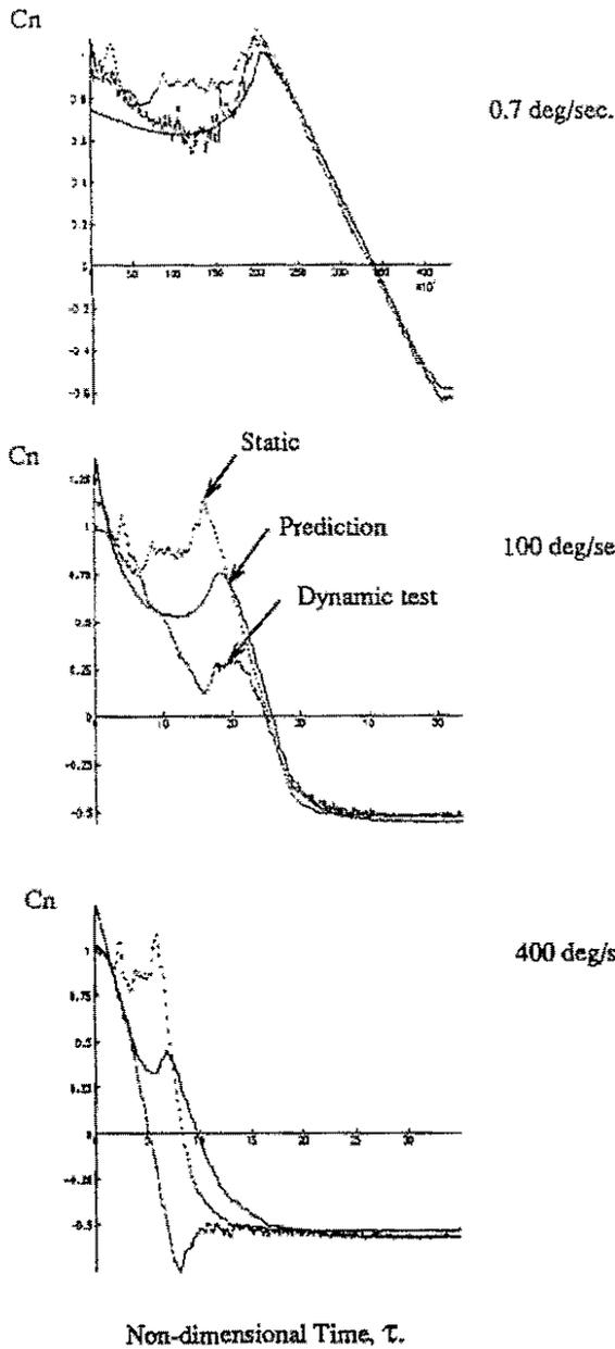
**Figure 12. Correlation of  $C_n$  from predictive method with wake modelling inclusion and test data.**
