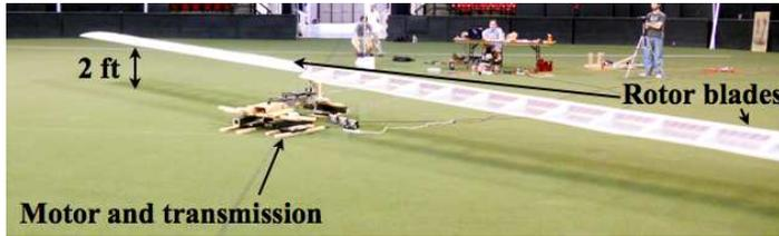
**Fig. 5: Full scale ground effect test rotor**
