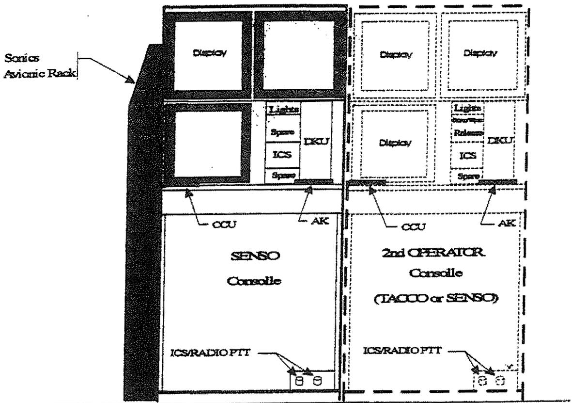
Figure 2: NH90 mission operator station(s) proposed lay-out
