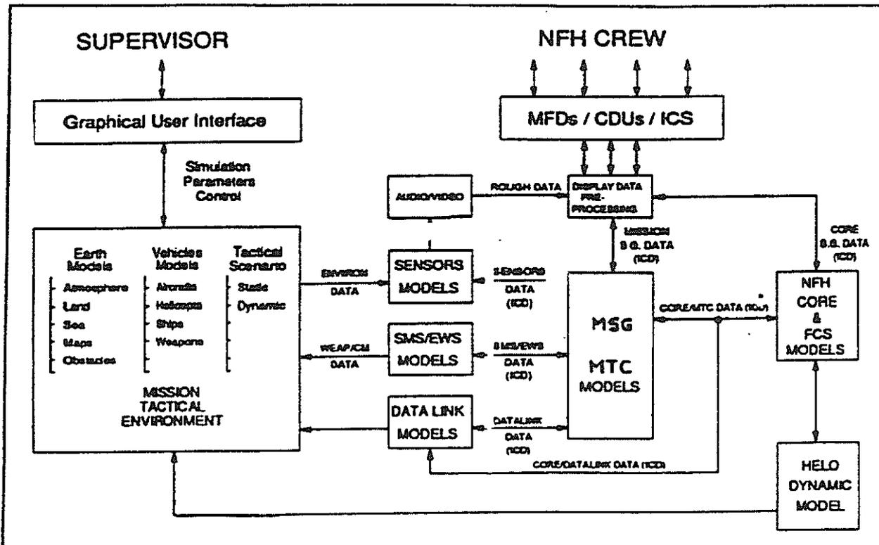
Figure 3: NH90 mission simulator functional architecture
