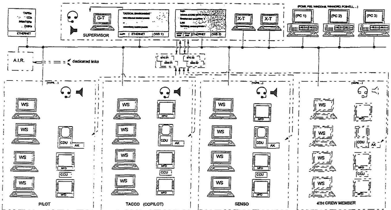
Figure 4: NH90 mission simulator hardware architecture
