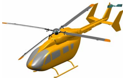
Figure 6 EC145 helicopter (CATIA v.4 model)
