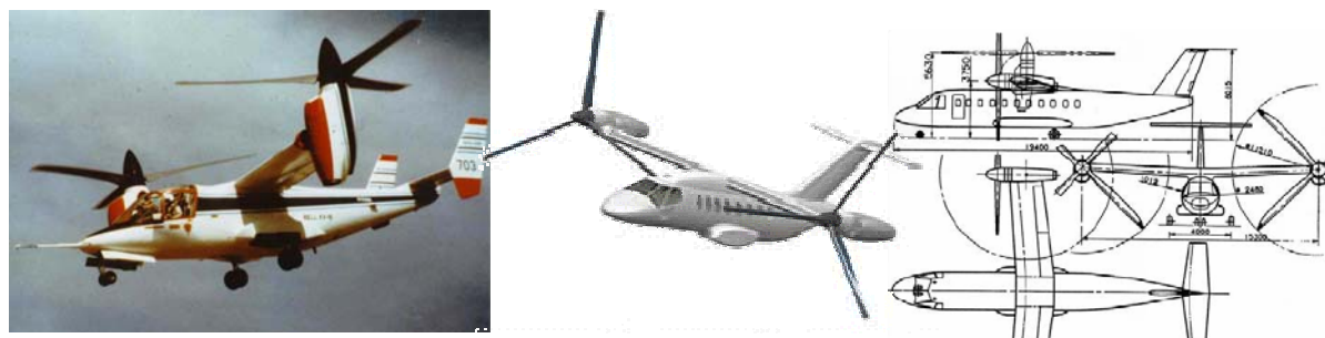
Figure 1 Bell-NASA-Army XV-15 Tilt Rotor and Eurocopter Eurotilt and Eurofar tilt rotor Concepts
