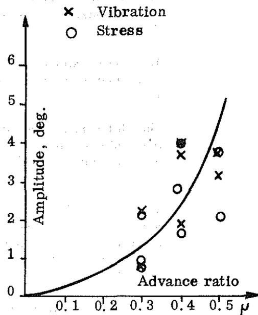
FIGURE 9 - PITCH AMPLITUDE DIVERGENCE
