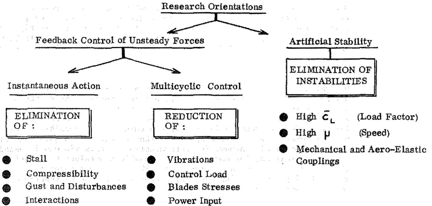
FIGURE 4 - ACTIVE CONTROL OF HELICOPTER ROTORS
