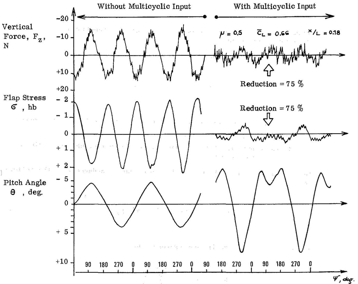
FIGURE 10 - EXAMPLE OF SIMULTANEOUS REDUCTION OF STRESS AND VIBRATION
