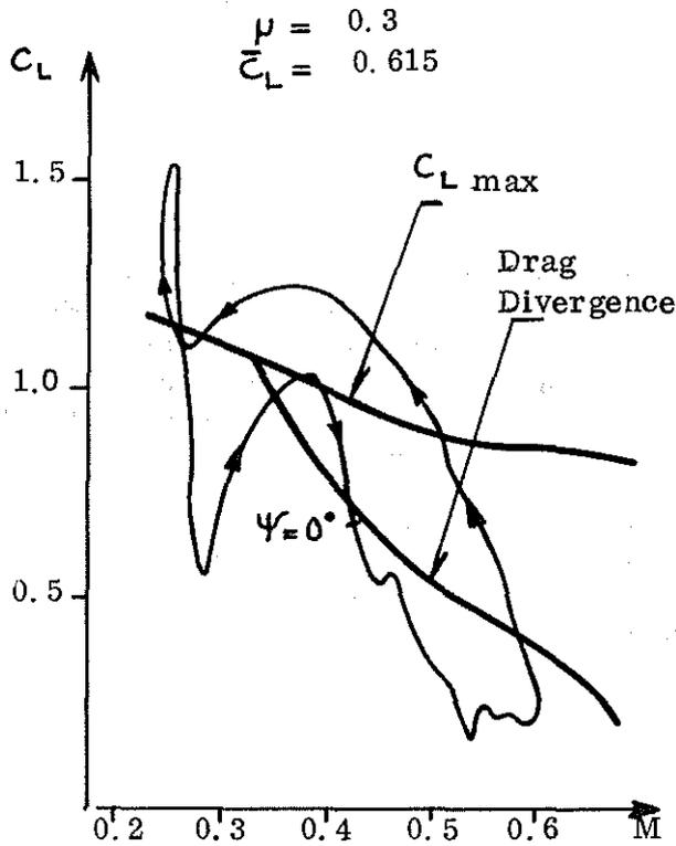
FIGURE 2 - WORKING CONDITIONS OF A ROTOR BLADE ELEMENT AT 0.71 RADIUS - REF. : 10
