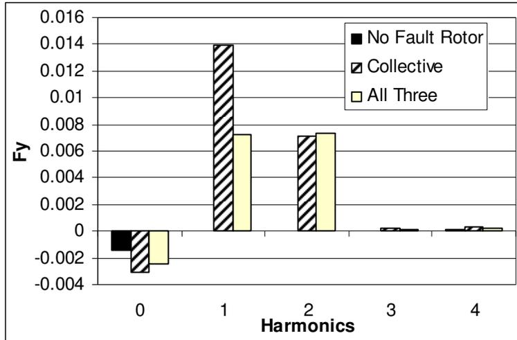
Figure 32 Lateral hub force of rotor with and without fault
