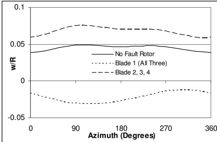
Figure 26 Tip flap response of rotor blades with and without "all three" fault
