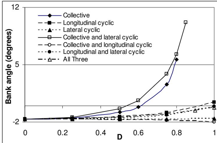
Figure 24 Effect of actuator damage on helicopter bank angle at  $\mu=0.3$
