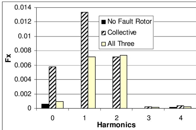
Figure 31 Longitudinal hub force of rotor with and without fault
