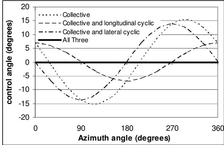
Figure 19 Control angle experienced by the blade with actuator damage at  $\mu=0.3$
