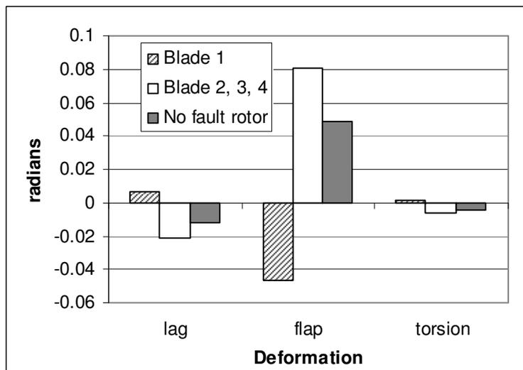
Figure 2 Steady tip deflections of no fault rotor, and damaged (blade 2, 3, and 4) and blades without actuator damage (blade 1) of rotor with fault in hover
