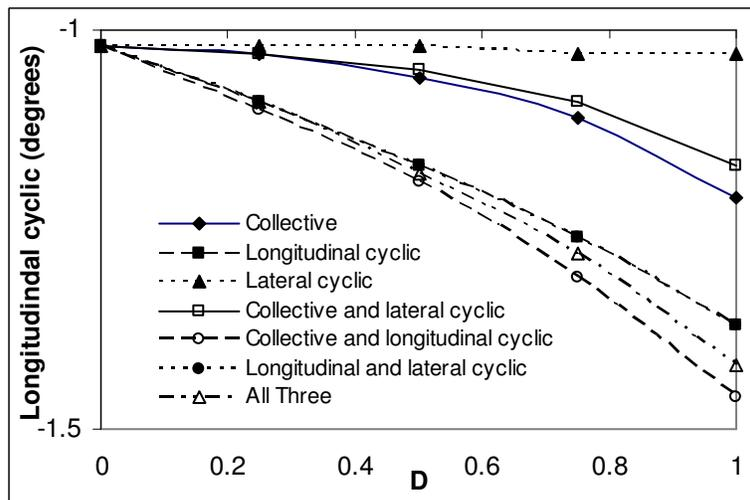
Figure 5 Effect of actuator damage on longitudinal cyclic of blades without actuator damage at  $\mu=0.1$
