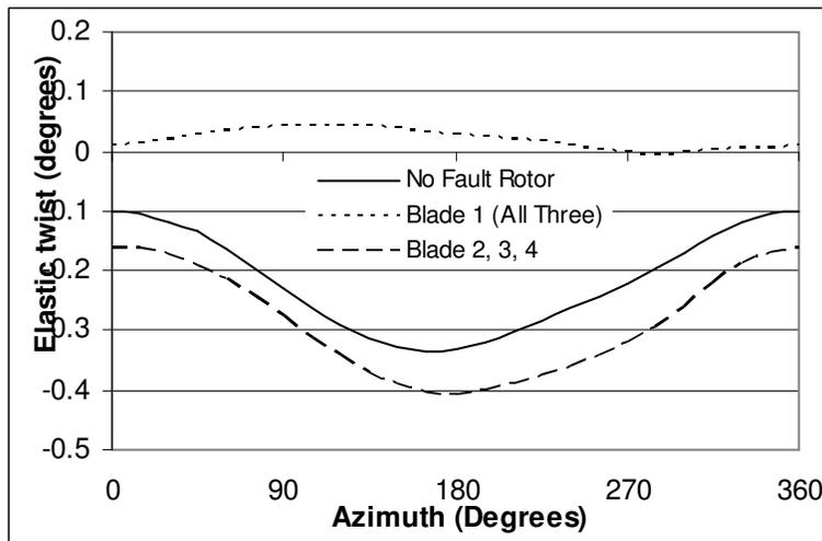
Figure 30 Tip elastic twist response of rotor blades with and without "all three" fault
