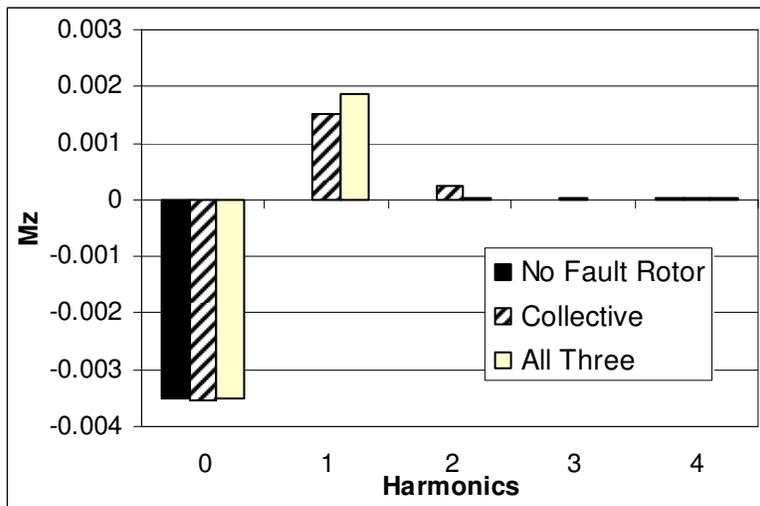
Figure 36 Hub yawing moment with and without faults
