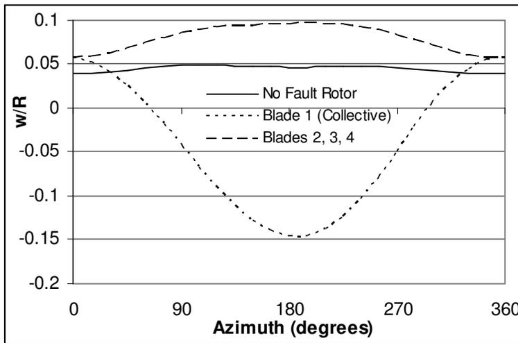
Figure 25 Tip flap response of rotor blades with and without collective fault
