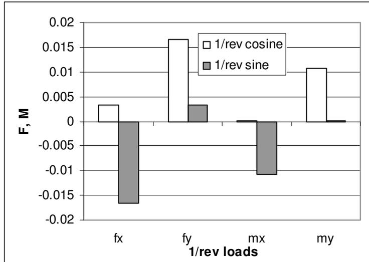
Figure 3 One per rev loads for rotor with actuator fault in hover
