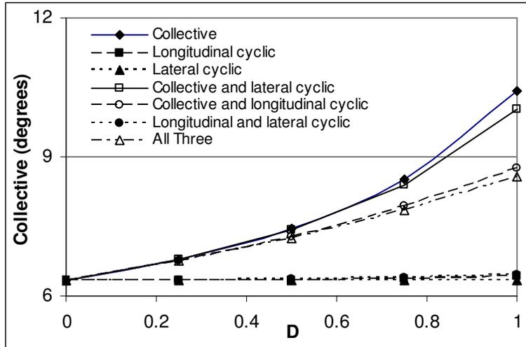
Figure 10 Effect of actuator damage on collective of blades without actuator damage at  $\mu=0.2$
