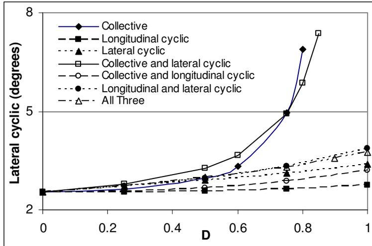
Figure 21 Effect of actuator damage on lateral cyclic of blades without actuator damage at  $\mu=0.3$
