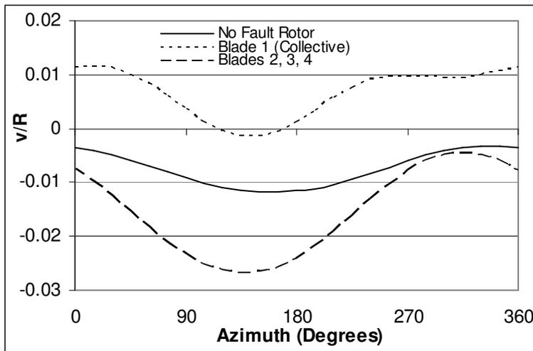
Figure 27 Tip lag response of rotor blades with and without collective fault
