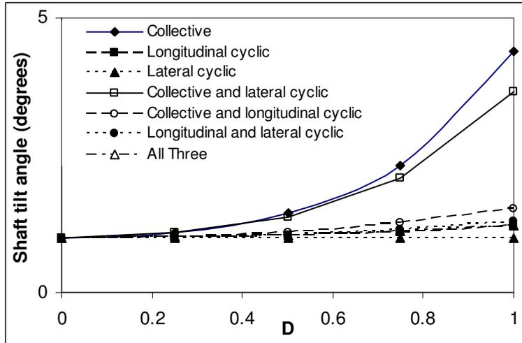
Figure 14 Effect of actuator damage on shaft tilt at  $\mu=0.2$
