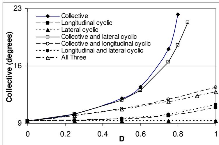
Figure 16 Effect of actuator damage on collective of blades without actuator damage at  $\mu=0.3$
