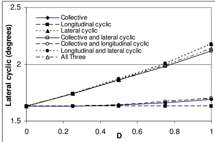
Figure 6 Effect of actuator damage on lateral cyclic of blades without actuator damage at  $\mu=0.1$
