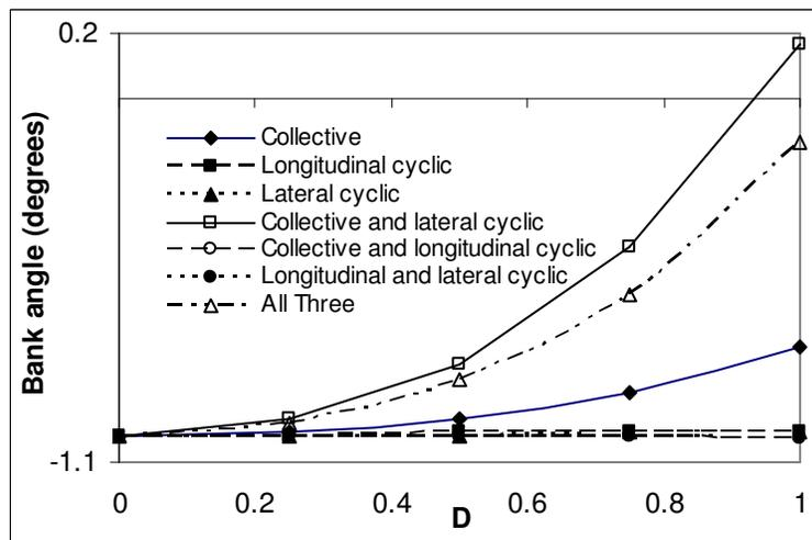
Figure 15 Effect of actuator damage on bank angle at  $\mu=0.2$
