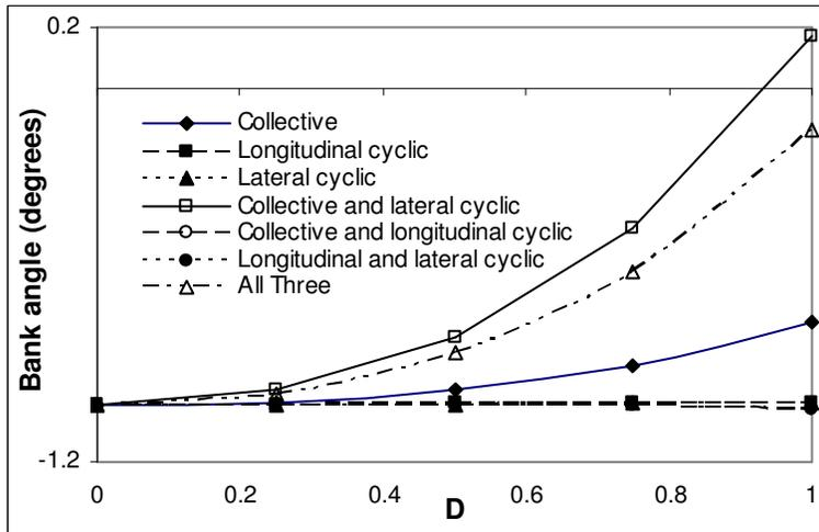
Figure 9 Effect of actuator damage on bank angle of helicopter at  $\mu=0.1$
