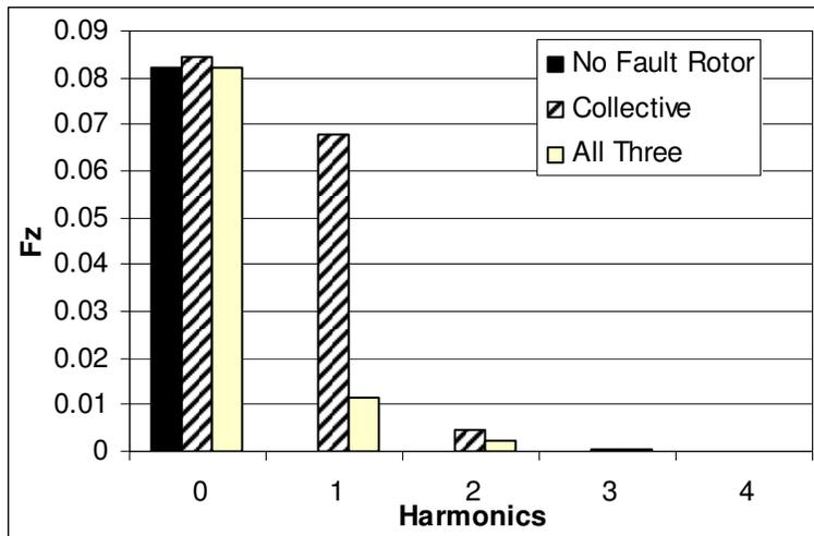
Figure 33 Vertical hub force of rotor with and without fault
