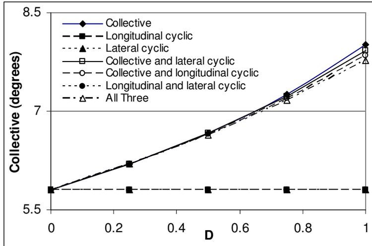
Figure 4 Effect of actuator damage on collective pitch of blades without actuator damage at  $\mu=0.1$
