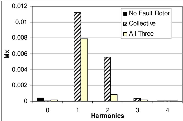
Figure 34 Hub rolling moment of rotor with and without fault
