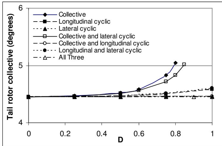
Figure 22 Effect of actuator damage on tail rotor collective at  $\mu=0.3$
