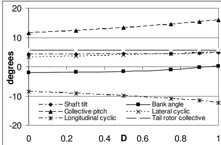
Figure 37 Trim control and vehicle attitude angles for reconfigured rotor with the “all three” fault at  $\mu=0.35$
