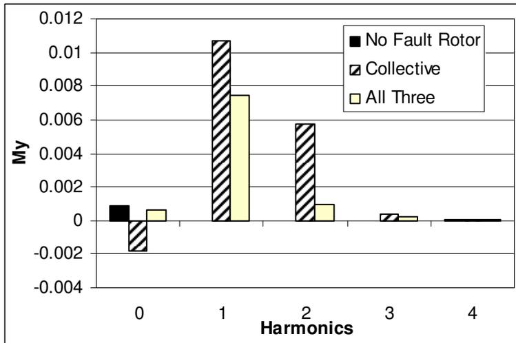
Figure 35 Hub pitching moment with and without faults
