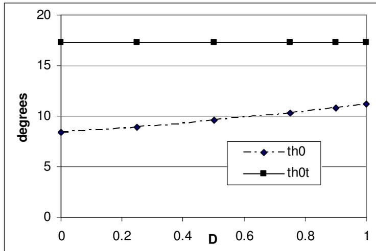
Figure 1 Effect of collective actuator damage on one blade on the collective pitch of blades without actuator damage and tail rotor collective in hover
