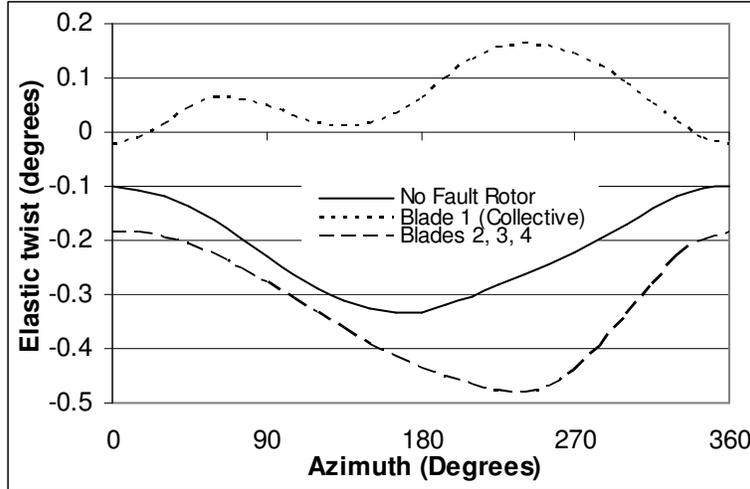
Figure 29 Tip elastic twist response of rotor blades with and without collective fault
