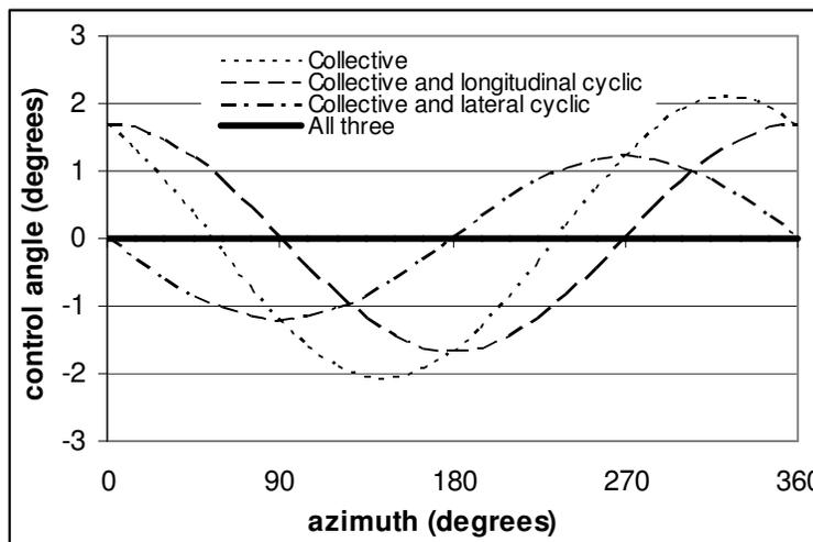
Figure 17 Control angle experienced by blade with actuator damage at  $\mu=0.1$
