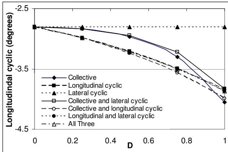
Figure 11 Effect of actuator damage on longitudinal cyclic of blades without actuator damage at  $\mu=0.2$
