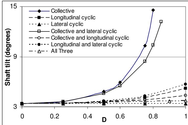
Figure 23 Effect of actuator damage on helicopter shaft tilt at  $\mu=0.3$
