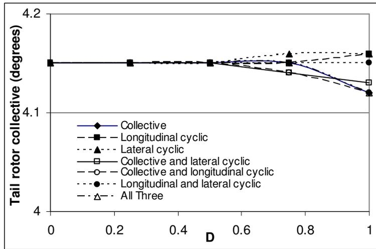
Figure 7 Effect of actuator damage on tail rotor collective at  $\mu=0.1$
