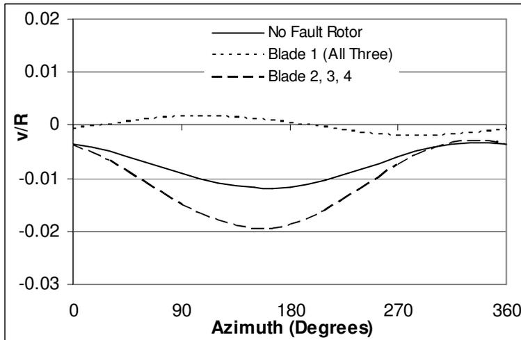
Figure 28 Tip lag response of rotor blades with and without "all three" fault
