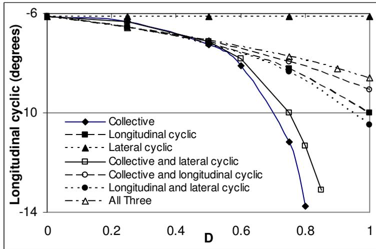
Figure 20 Effect of actuator damage on longitudinal cyclic of blades without actuator damage at  $\mu=0.3$
