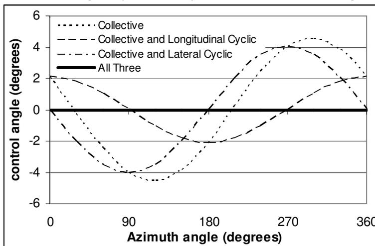
Figure 18 Control angle experienced by blade with actuator damage at  $\mu=0.2$
