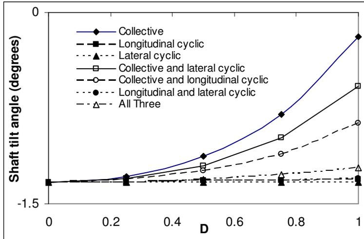
Figure 8 Effect of actuator damage on shaft tilt angle of helicopter at  $\mu=0.1$
