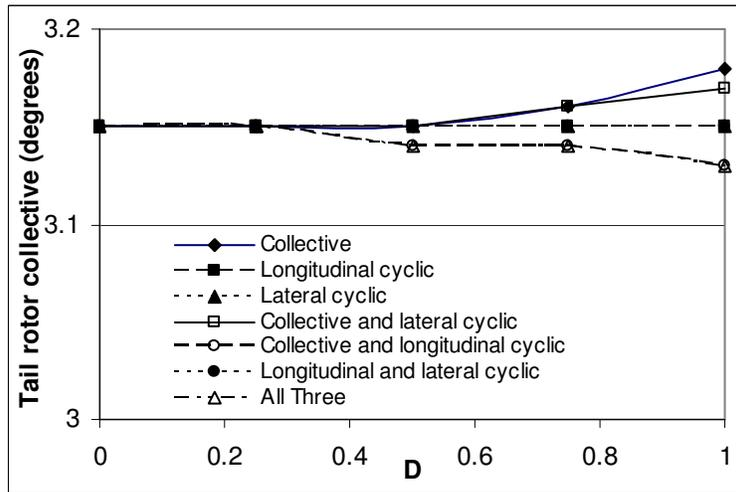
Figure 13 Effect of actuator damage on tail rotor collective at  $\mu=0.2$
