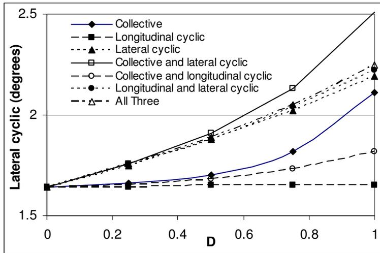
Figure 12 Effect of actuator damage on lateral cyclic of blades without actuator damage at  $\mu=0.2$
