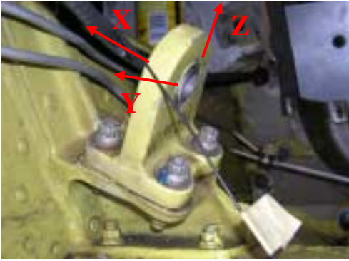
Figure 2: local coordinate system on a strut
