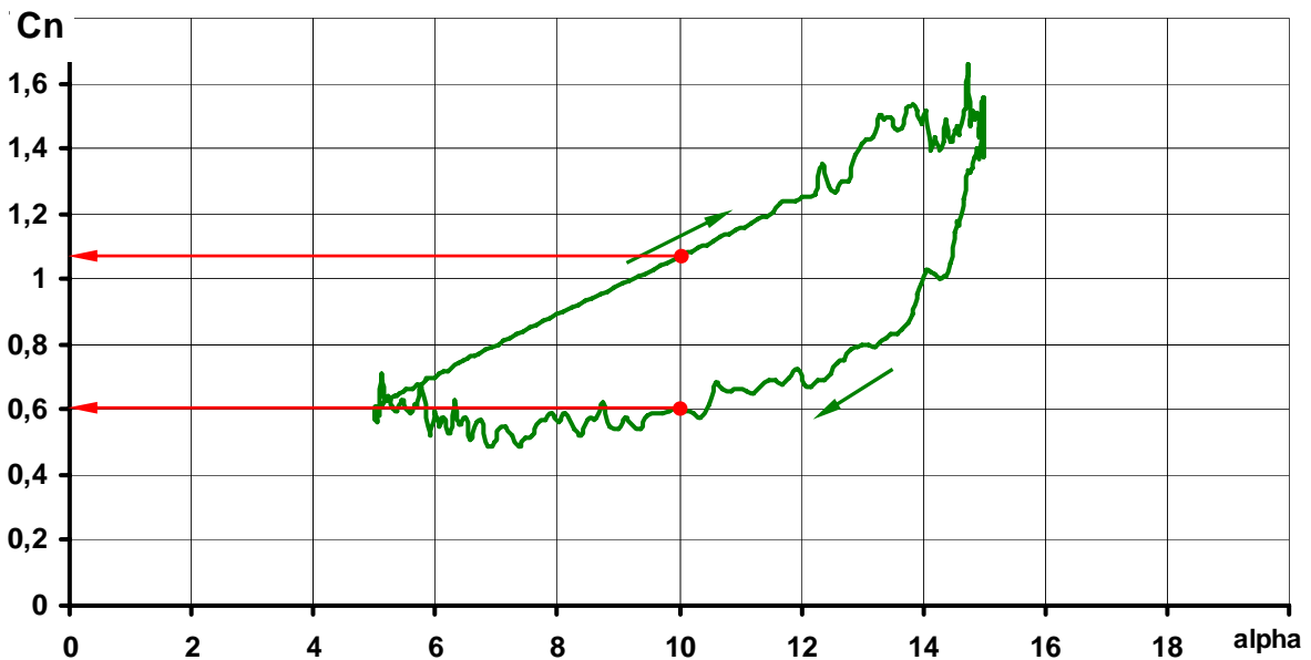
Figure 12. Normal force coefficient versus angle of attack curve for the harmonically oscillating airfoil at Sh = 0,25
