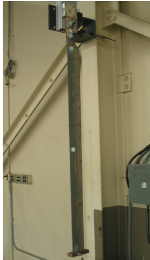
Fig. 2 Measurement of the flap bending for HART I blade with the mirror method.
