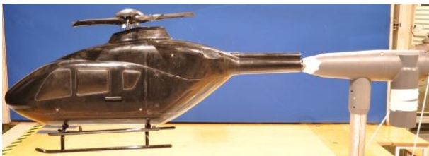
Fig. 5. Baseline configuration of the ADHeRo wind tunnel model (F0M0L0R0).
