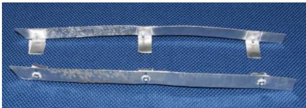
Fig. 13. Sheet metal type strakes with mounting brackets.
