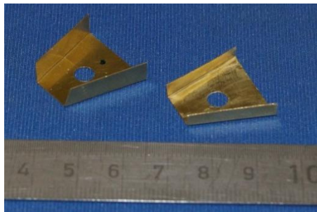
Fig. 10. Vortex generator wind tunnel models made from brass sheet metal of 0.2 mm thickness. Specimen tested in wind tunnel: left) boundary-layer-scaled VG, right) sub-boundary-layer VG.
