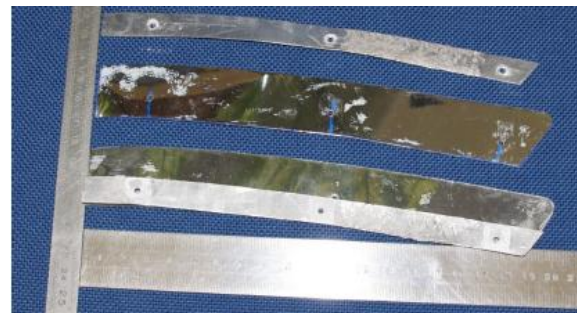
Fig. 16. Different plan form geometries for the sheet metal type strakes. Top: Plan form (b), Centre: Plan form (a), Bottom: Both plan forms in direct comparison.
