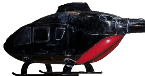
Fig. 12. Contoured strakes cast silicon parts (red) installed on the ADHeRo wind tunnel model
