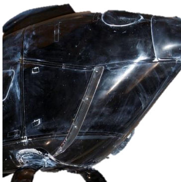
Fig. 14. Simple strake S1 installed at the wind tunnel model.
