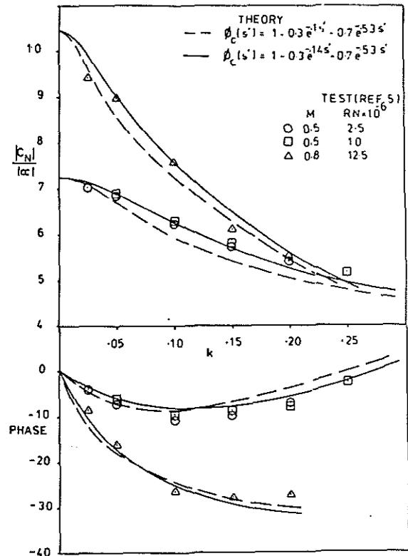
FIG. 5. FREQUENCY RESPONSE COMPARISON
