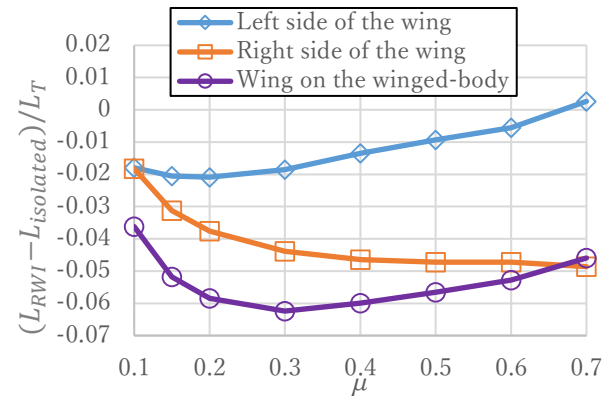
Fig. 14 The influence to the lift on the parts of the wing on the winged-body focusing on aerodynamic characteristics of an aircraft. (nondimensionalized by the total lift.)
