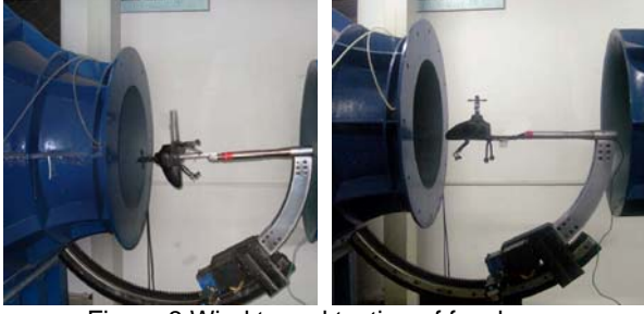
Figure 3 Wind tunnel testing of fuselage
