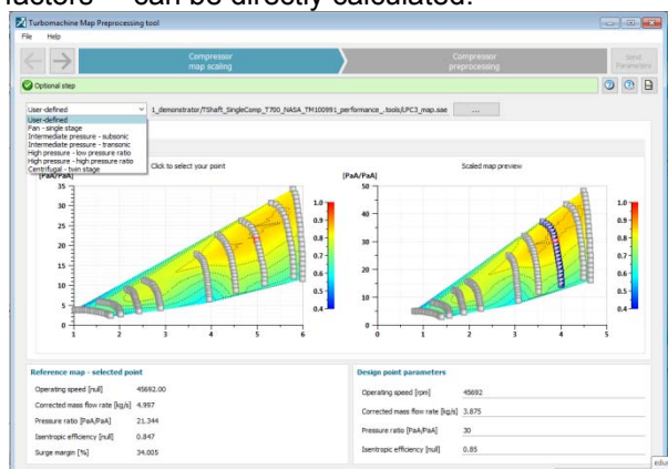
Figure 2: Compressor Map scaling tool
