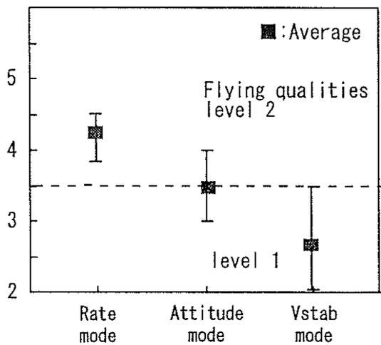
Figure.13 Pilot Rating of Low-speed climb and descent in IMC
