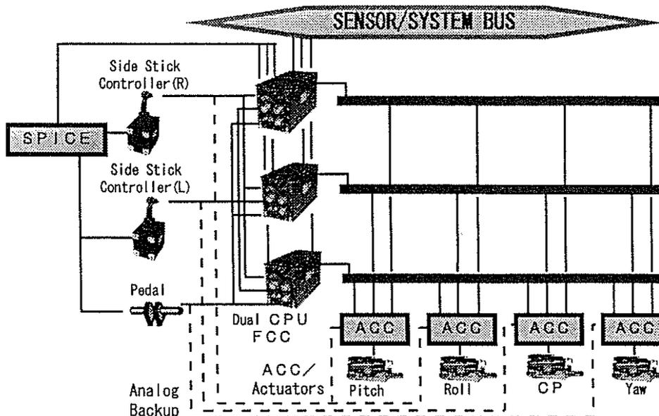
Figure.2 Configuration of the flight control system
