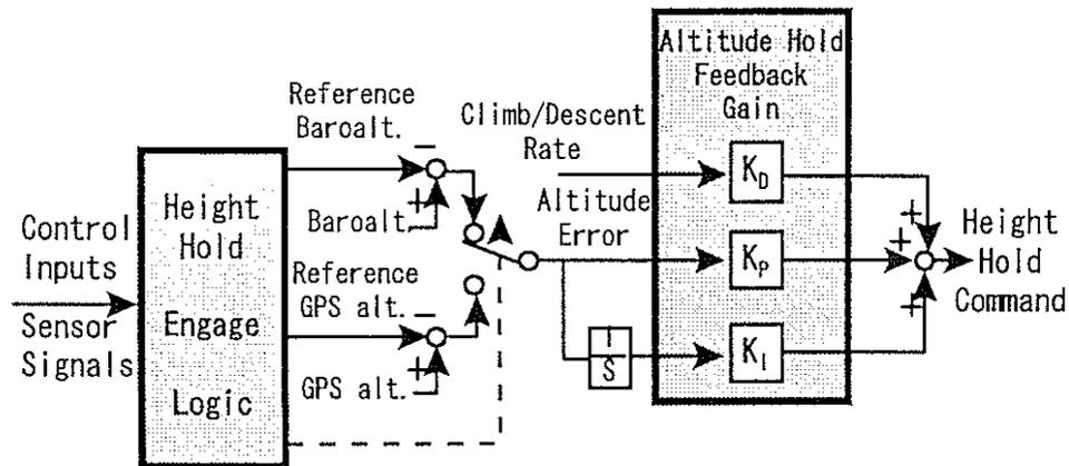
Figure.6 Block diagram of Hold Function
