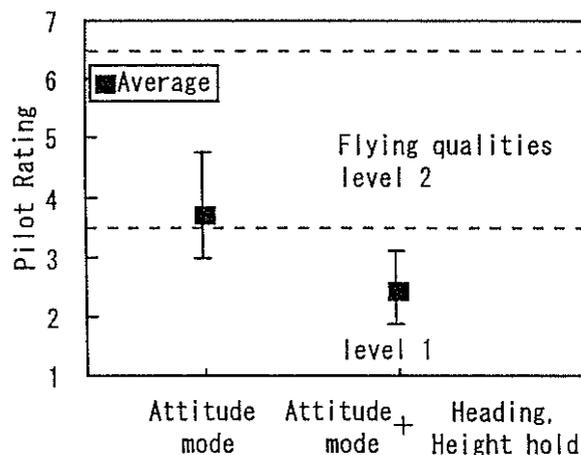
Figure.15 Pilot Rating of Low-speed flight task in IMC with and without Hold Function
