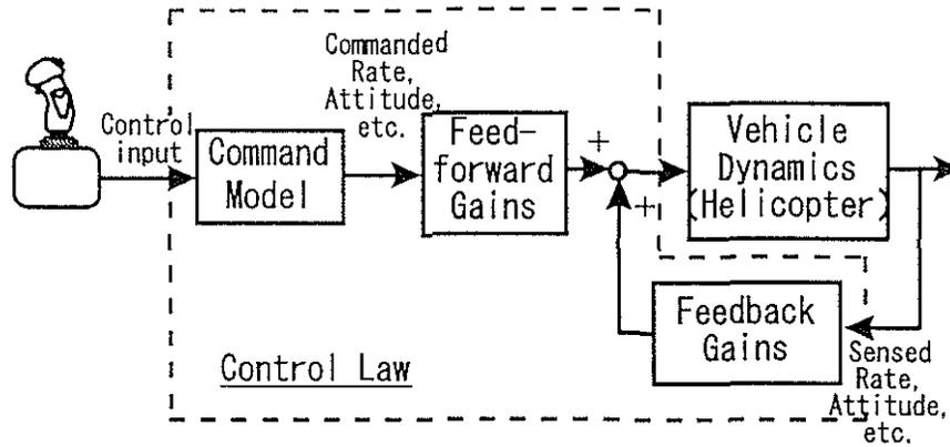
Figure.4 Configuration of the Core Function
