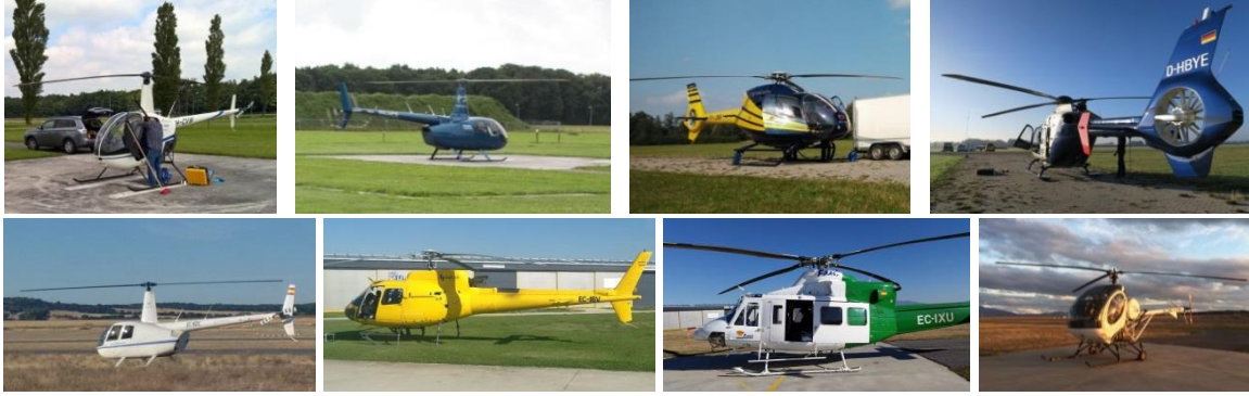
Figure 4 Helicopter types selected for noise measurements (top, left to right): Robinson R22 and R66, Eurocopter EC120 and EC135; (bottom) Robinson R44, Airbus Helicopters AS350, Bell B412 and Schweizer S300
