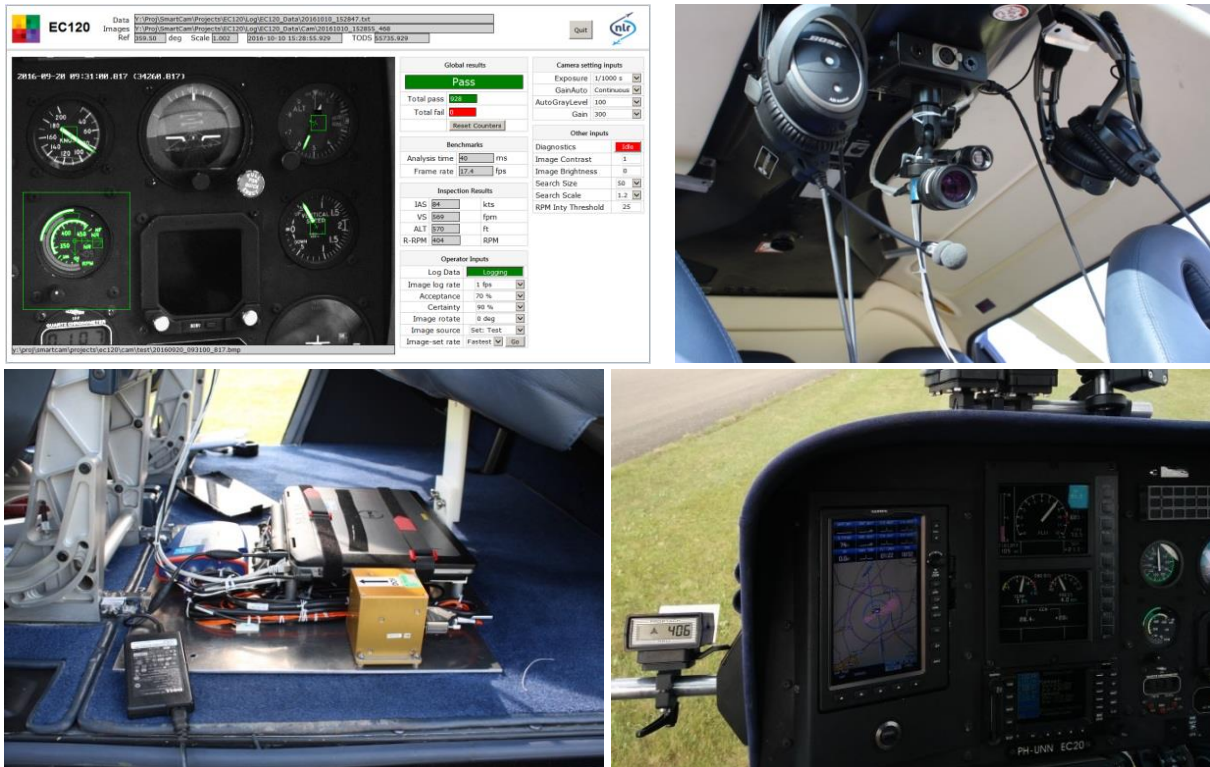
Figure 6 Carry-On Flight Data Recorder (COFDR): SmartCam digitization of performance indicators (top left); camera mounting (top right); Laptop, GNSS receiver and IMU (bottom left), EC120 instrument panel and optical tachometer (bottom right)
