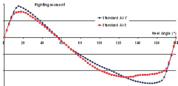
Fig. 4: Righting moment curves for the heaviest (red) and lightest (blue) mass configurations
