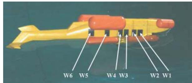
Fig. 8: Inverted model in waves.
