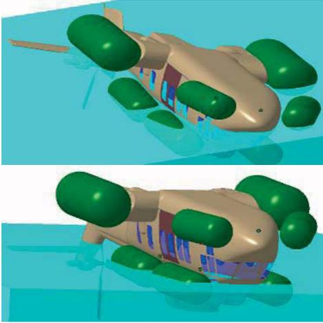
Fig. 6: EFS configurations C3. Equilibrium positions for load cases AV1 (top) and AV3 (bottom)
