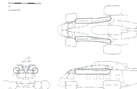
Fig 2: Long buoyancy bags along upper cabin.
