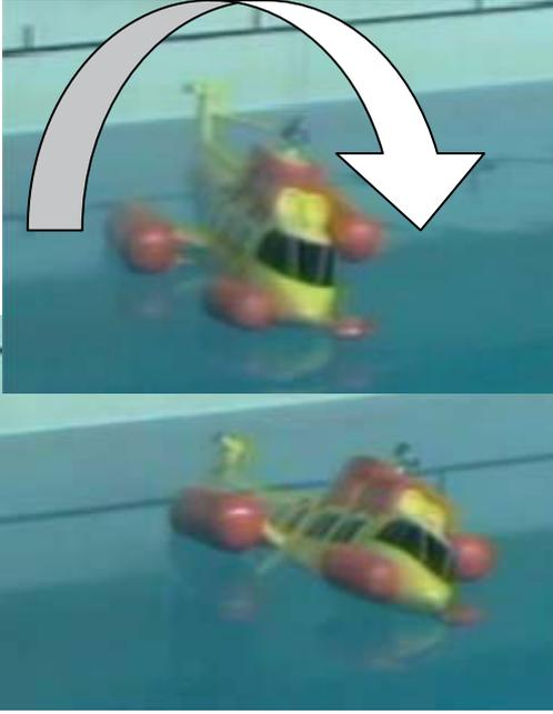
Fig. 11: Impact without one the standard rear port float for configuration 5
