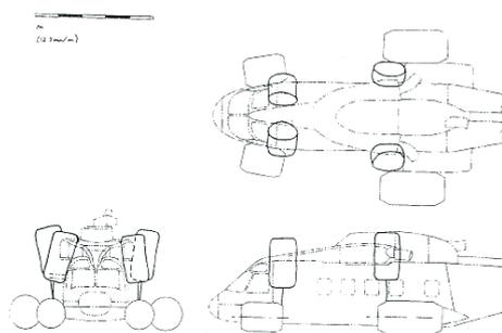
Fig. 3: Tethered inflatable floatation units
