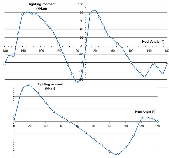
Fig. 7: Righting moment curves for EFS configuration 5 (top) and 6 (bottom)
