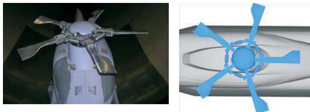
Figure 26: Experimental and numerical model with the mast, the blade sleeves, the lead-lag dampers, the pitch-rods, the rotor cap and the blade roots
