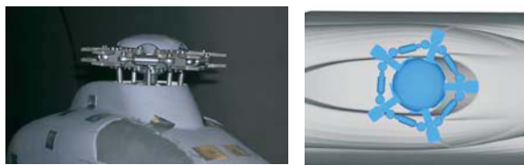
Figure 23: Experimental and numerical models of the mast with blade sleeves, lead-lag dampers and rotor cap installed on the fuselage
