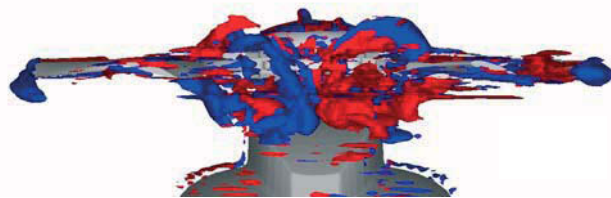
Figure 28: Wake emitted by the rotor hub
