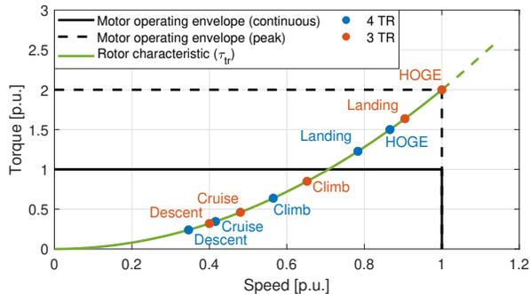
Figure 5: Motor operating points on rotor characteristic.
