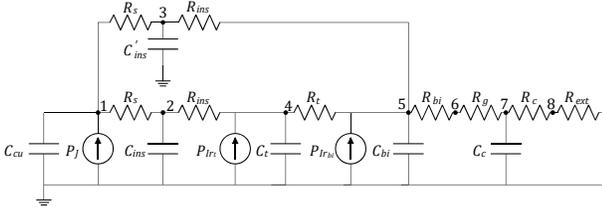
Figure 8: Motor lumped parameter thermal network.
