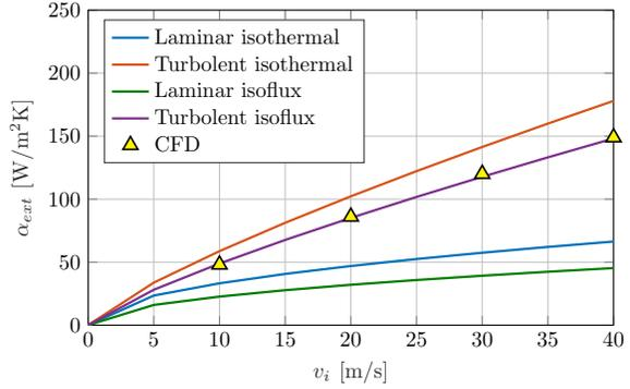
Figure 9: Convection coefficient correlations.
