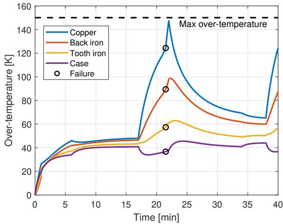
(b) Motor temperature rise, from 4 TR to 3 TR.
