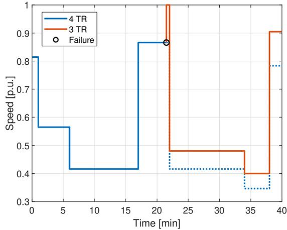
(a) Motor speed reference: from 4 TR to 3 TR.
