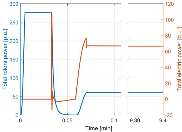
(a) Rotor vs motor (total) absorbed power.
