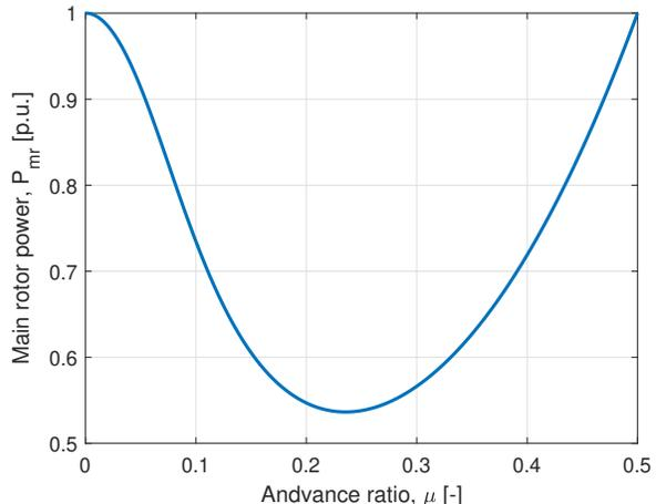
Figure 4: Main rotor power vs helicopter advance ratio.
