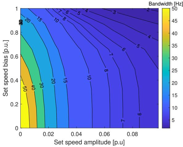
(b) Bandwidth contours vs set amplitude and bias.
