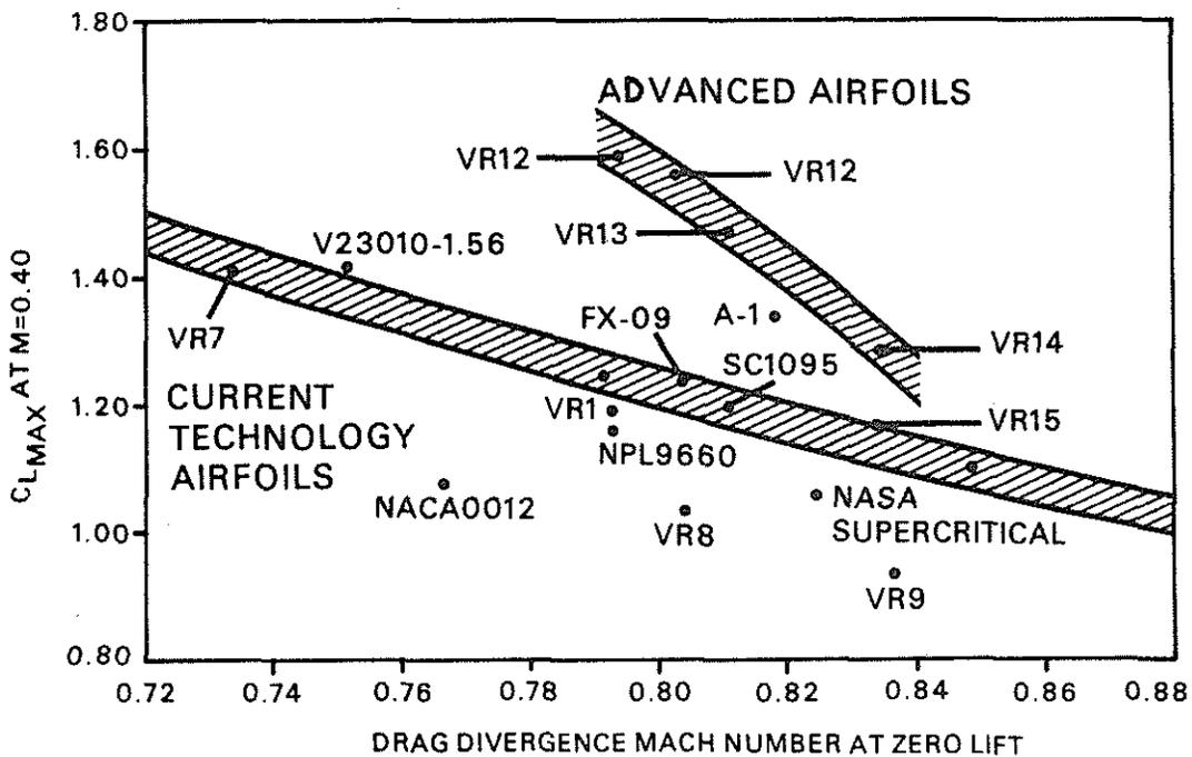
Figure 1. Comparison of rotor airfoil characteristics.
