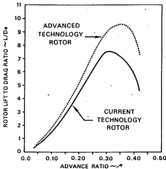
Figure 4. Helicopter rotor forward flight performance.
