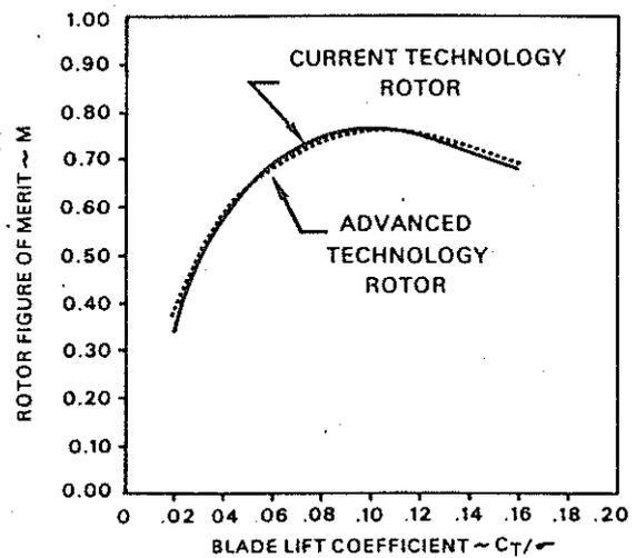
Figure 5. Helicopter rotor hover performance.
