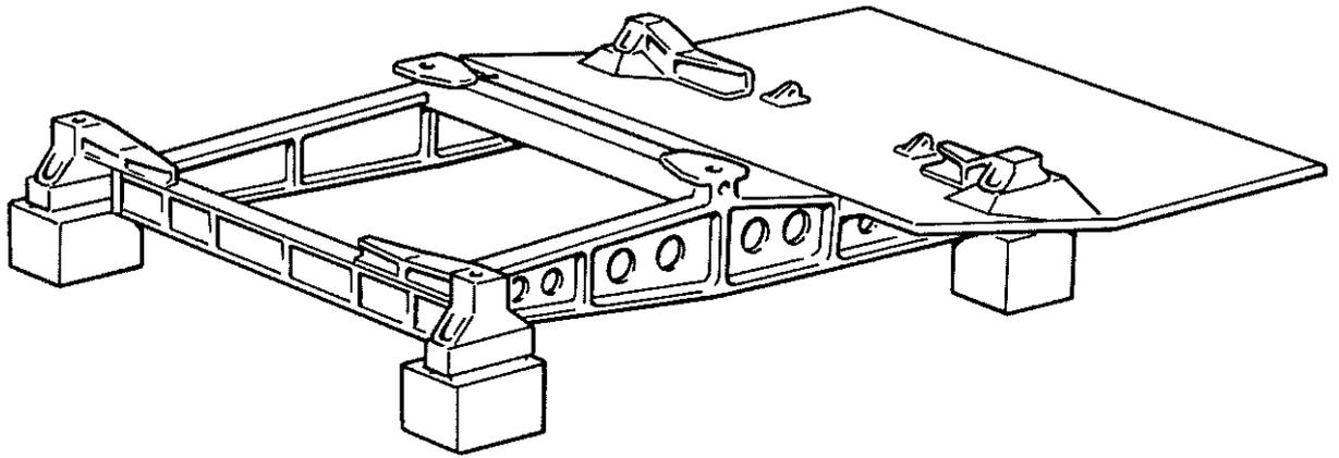
FIG.17. THE 4 POINT SUSPENSION RAFT SYSTEM
