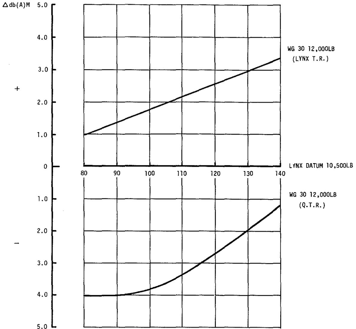
FIG.10. WG.30 EXTERNAL NOISE REDUCTION
