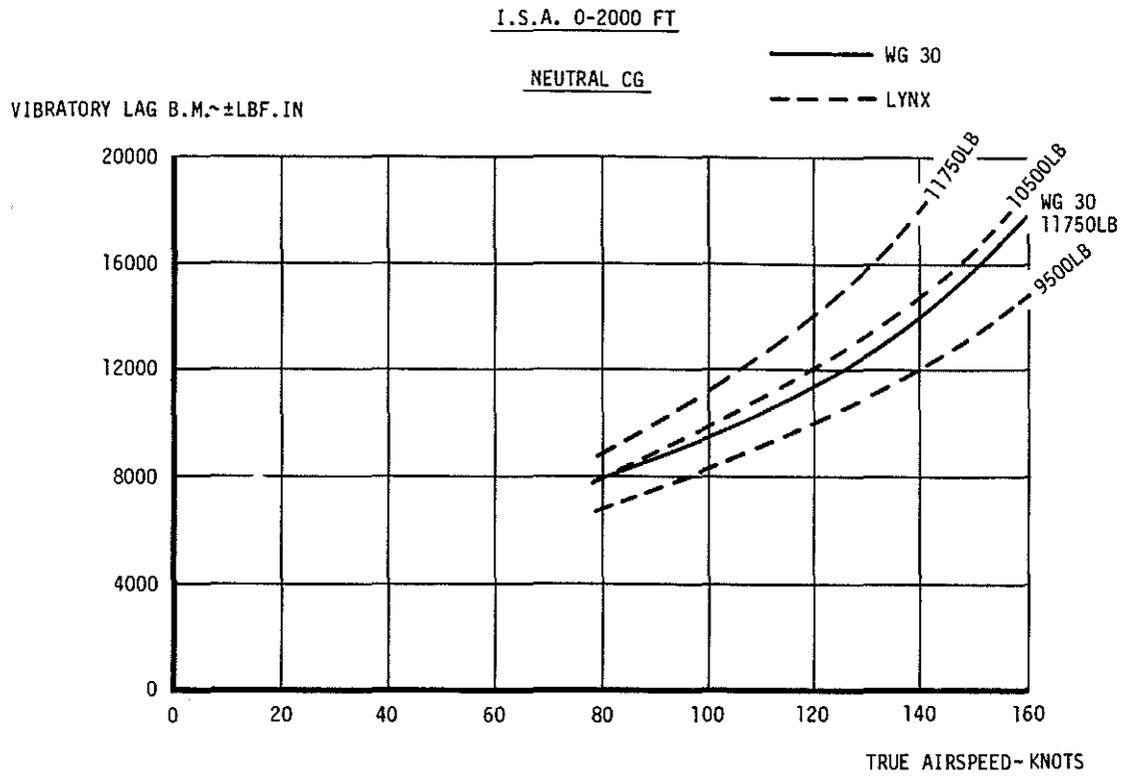
FIG.7. COMPARISON OF 31-0% ROTOR RADIUS LAG VIBRATORY LOADS WITH LYNX
