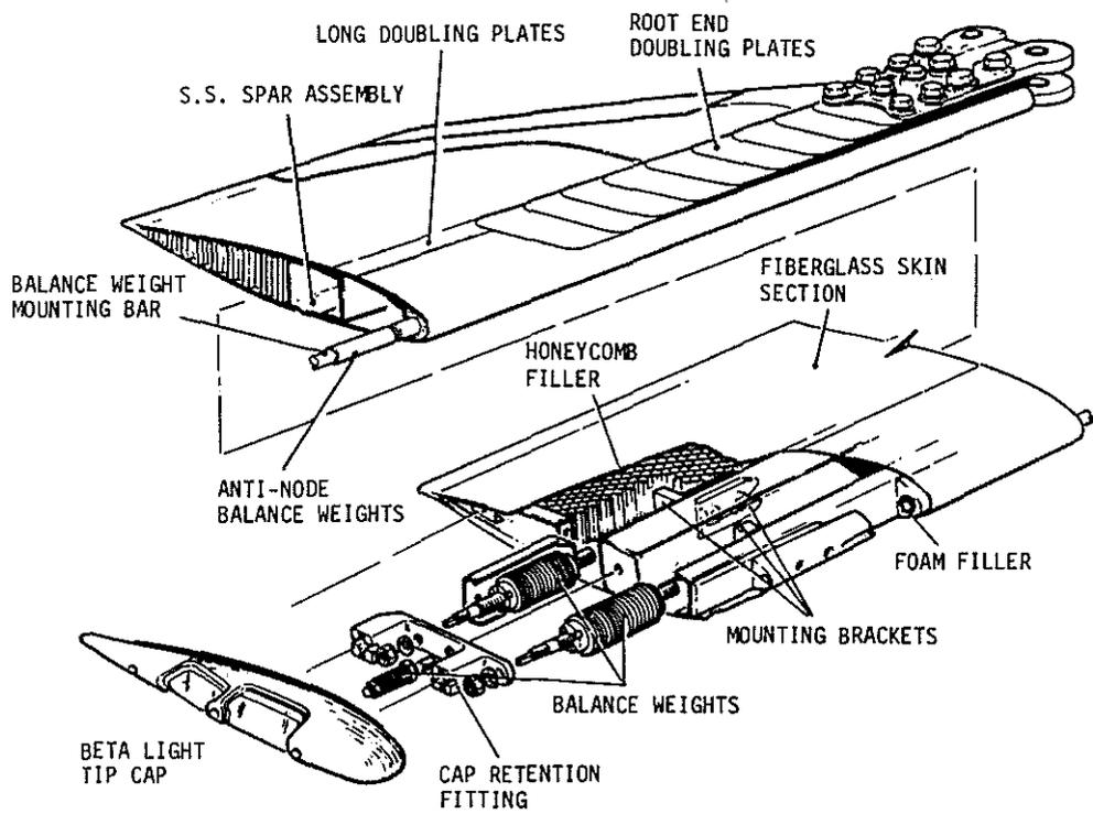
FIG.4. ROTOR BLADE TECHNOLOGY
