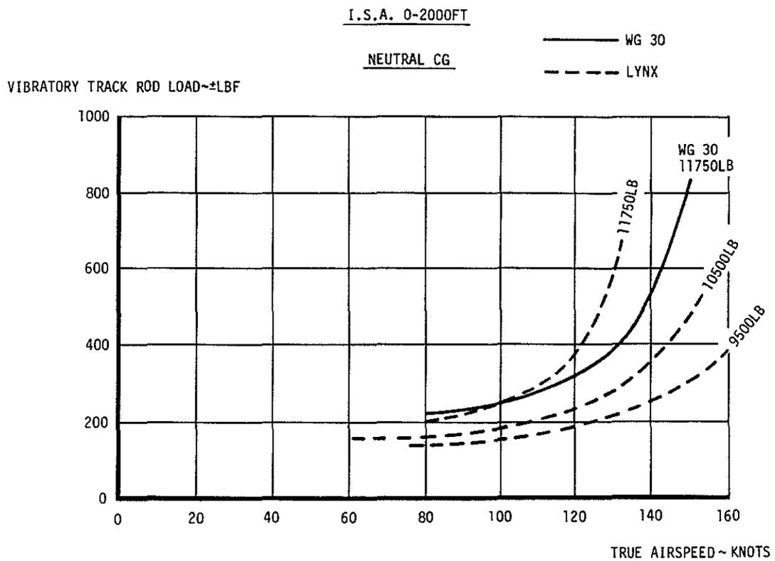
FIG.8. COMPARISON OF MAIN ROTOR TRACK ROD VIBRATORY LOADS WITH LYNX
