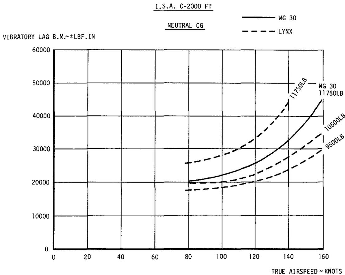
FIG.6. COMPARISON OF 6-8% ROT. RAD. LAG VIBRATORY LOADS WITH LYNX
