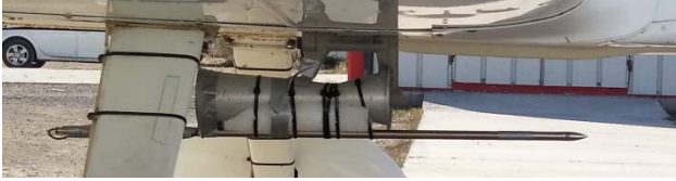
Figure 8: Boom microphone during Trebujena tests
