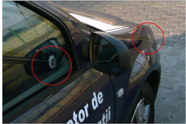
Figure 2: Microphone positions during highway tests
