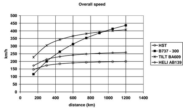
Figure 2 – Overall speed of airplane, train and rotorcraft
