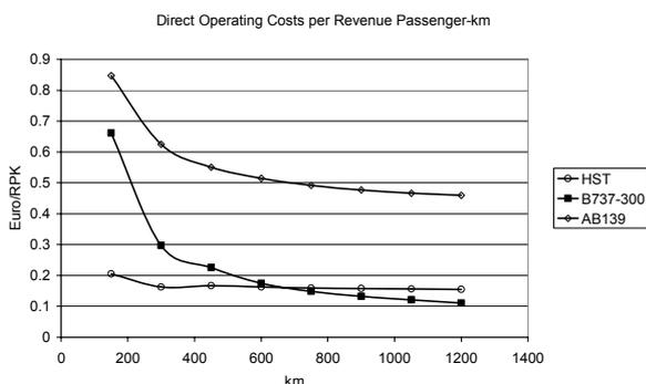
Figure 14 – Direct Operating Costs per Revenue Passenger-km
