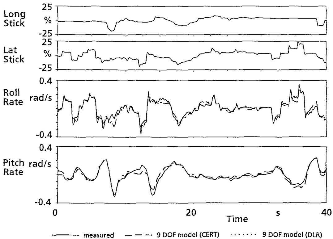
Figure 10. Comparison of the measured roll and pitch rates and the responses of the 9 DOF models identified by CERT and DLR for the first data run shown in Figures 5 and 6 (mainly lateral stick control inputs)
