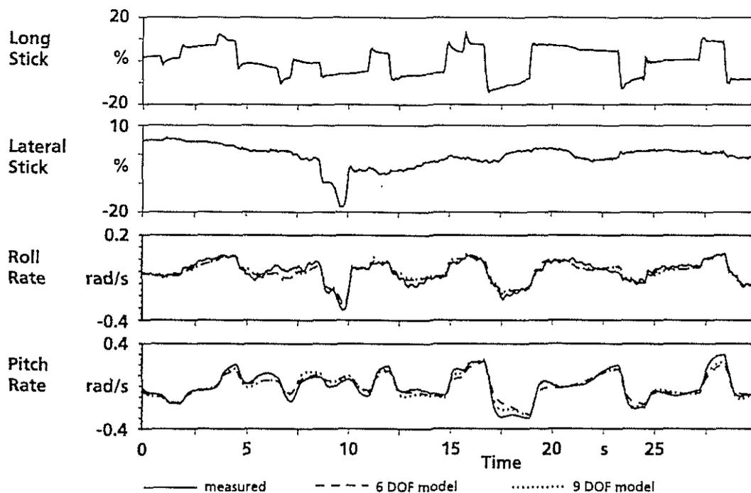
Figure 12. Comparison of the measured roll and pitch rates and the responses of the identified models with 6 and 9 DOF for the second data run with mainly longitudinal stick control inputs (flight data as in Figure 11)
