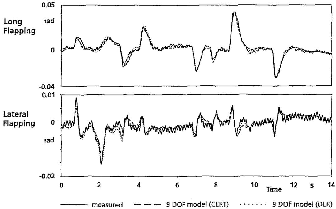
Figure 9. Comparison of the measured rotor response and the responses of the 9 DOF models identified by CERT and DLR for a representative data segment from the first data run shown in Figures 5 and 6 (from 14 to 28 seconds)
