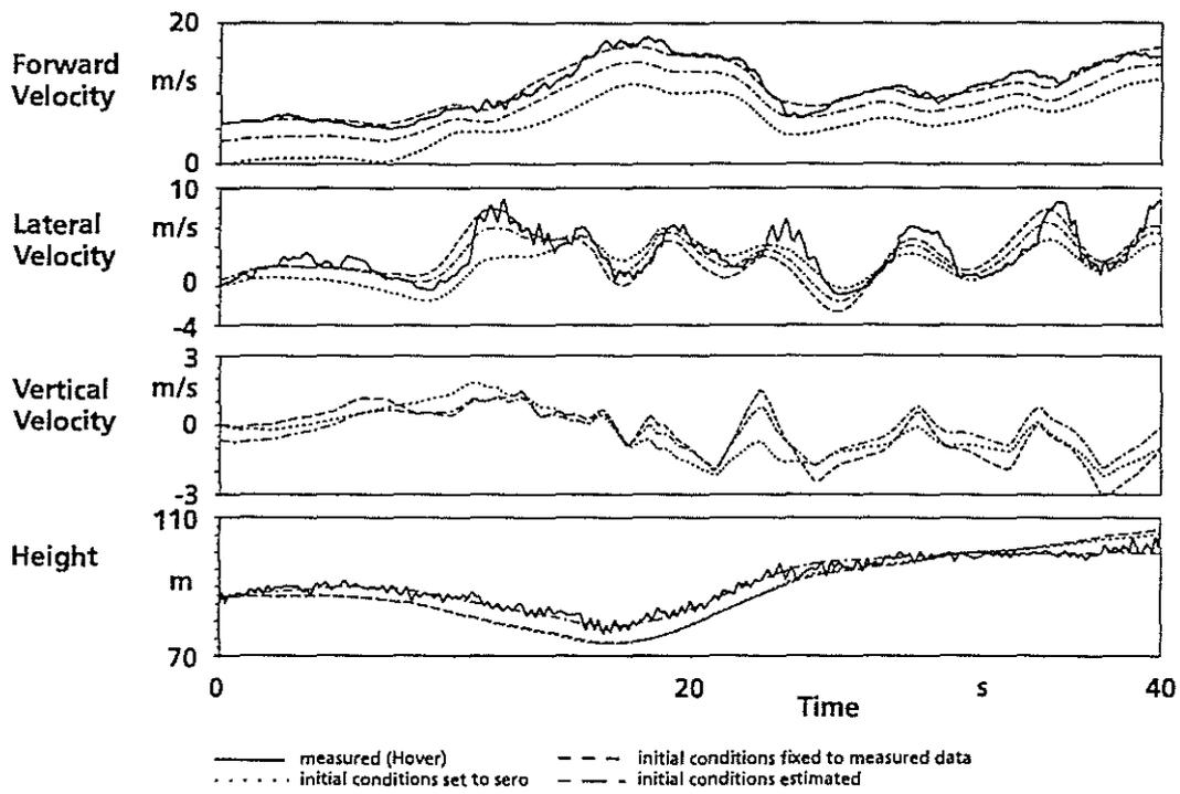
Figure 4. Velocity reconstruction and its sensitivity to initial conditions
