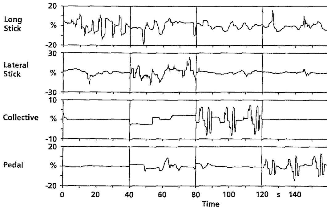
Figure 5. Control inputs of the common data set selected for the identification
