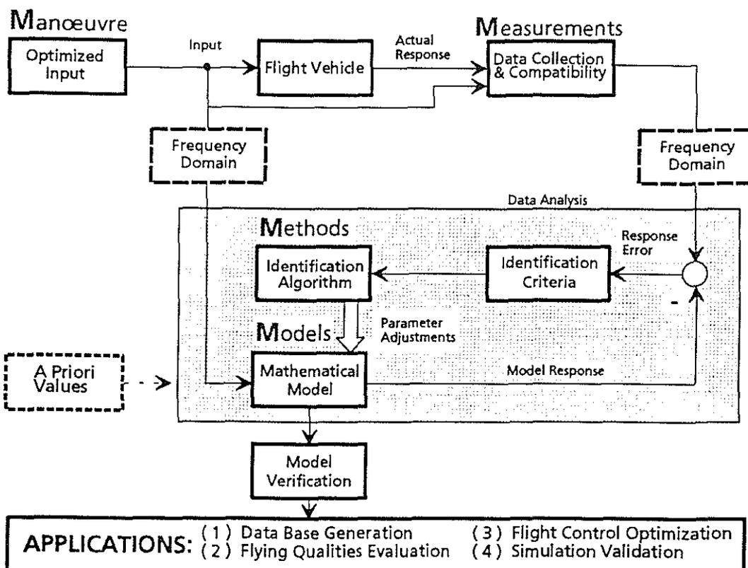
Figure 1. Principal approach for system identification
