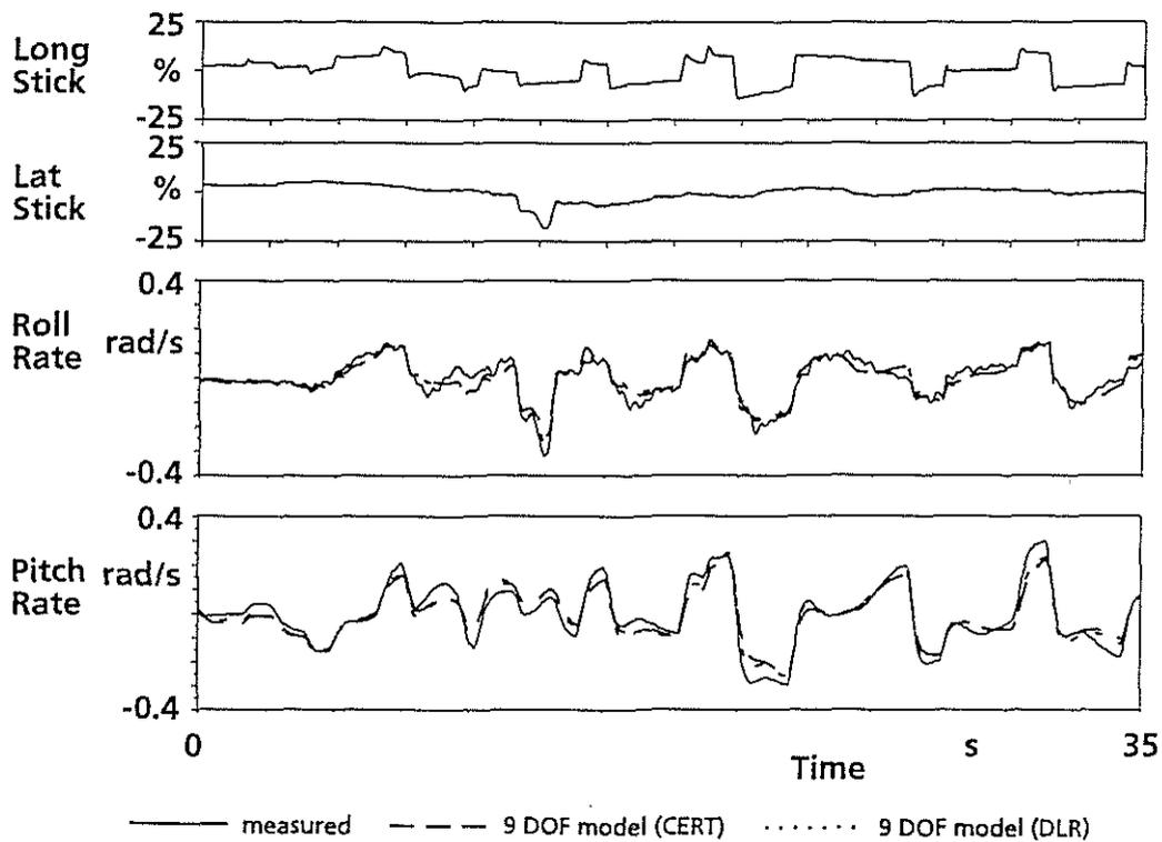
Figure 11. Comparison of the measured roll and pitch rates and the responses of the 9 DOF models identified by CERT and DLR for the second data run shown in Figures 5 and 6 (mainly longitudinal stick control inputs)
