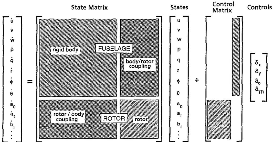
Figure 7. Principle of extended model structure
