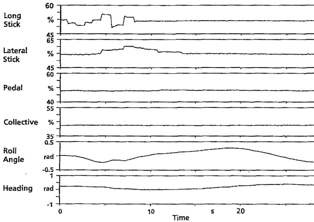
Figure 2. System identification control inputs for 80 knots flight condition and roll and heading response
