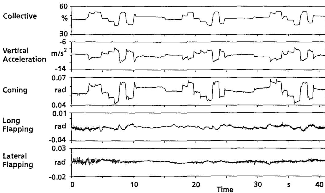
Figure 8. Rotor data quality check: measured rotor response due to collective inputs and correlation of the coning and vertical acceleration data
