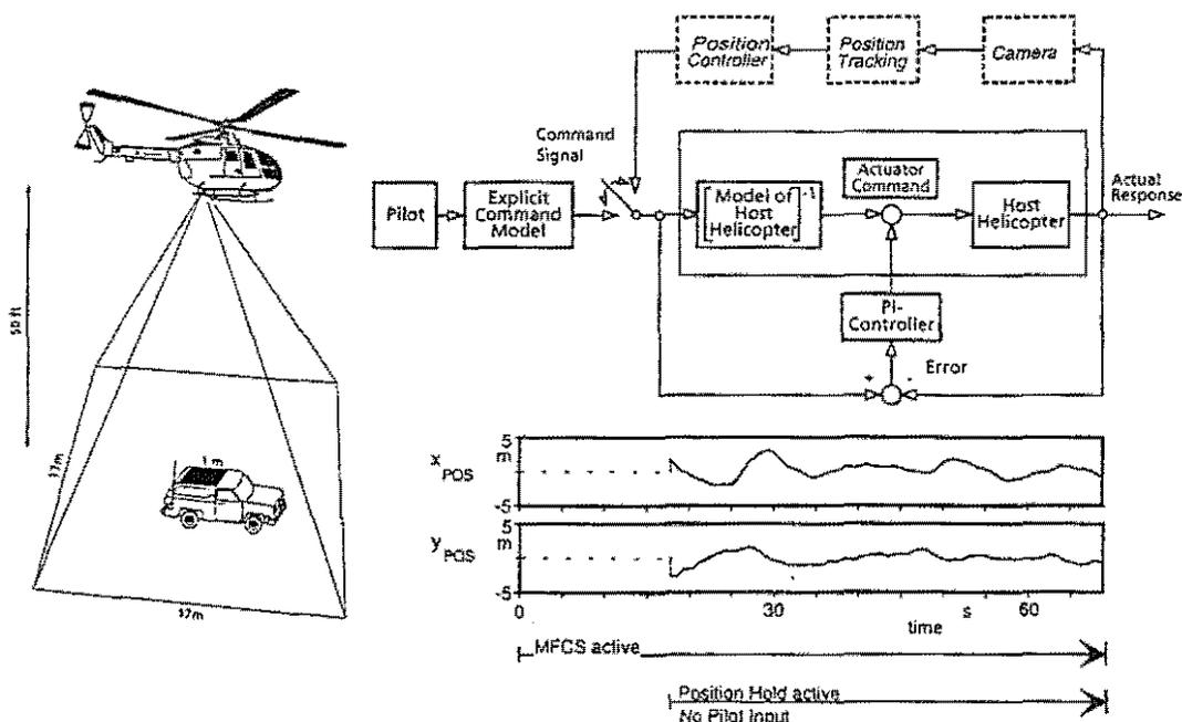
Figure 14. Application of the identified extended model for the control system design for In-Flight Simulation: Principle of In-Flight Simulation with additional feedback for an automatic position hold tracking task, Flight test set up, and results for a position hold over a car, moving in a full circle.
