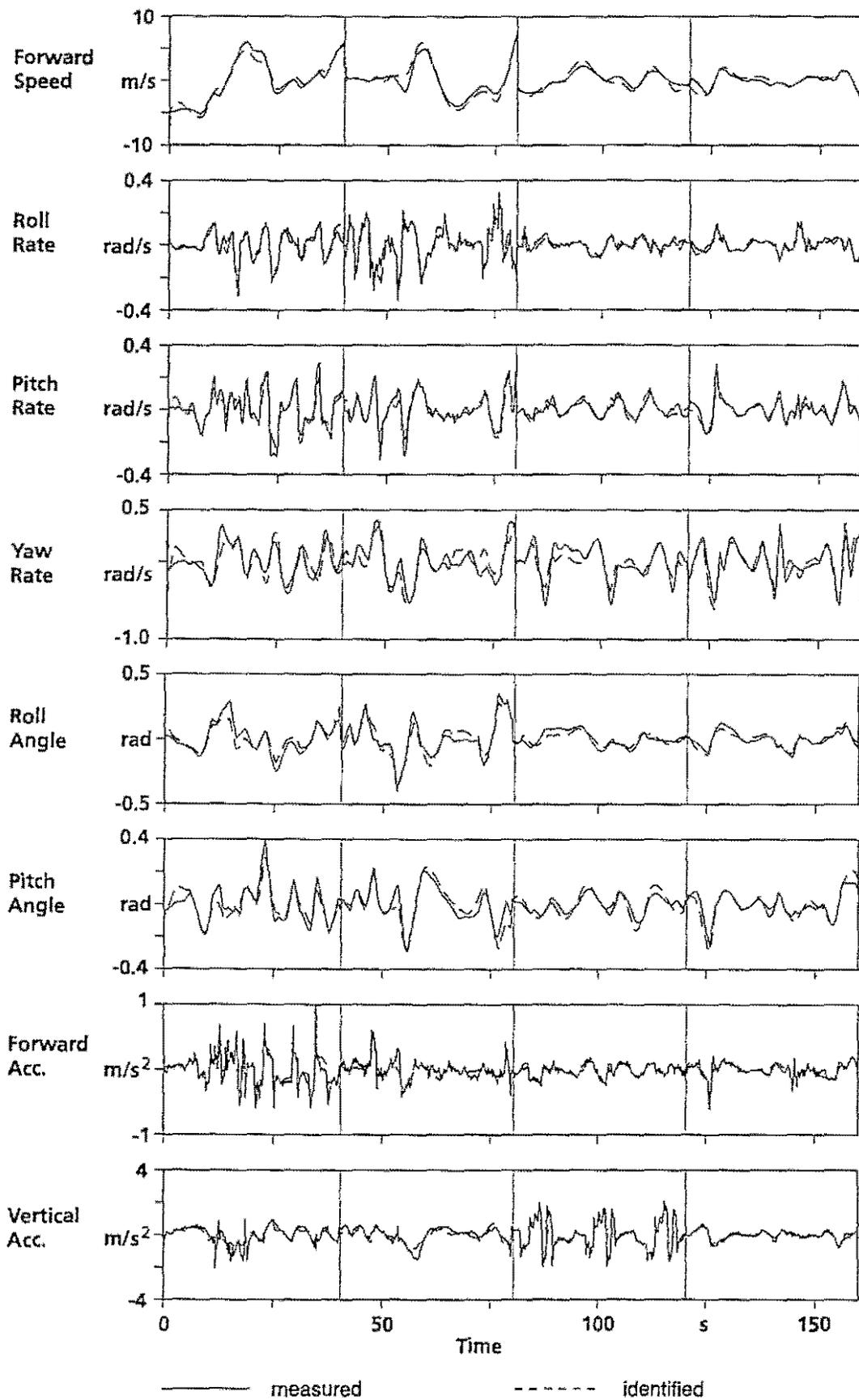
Figure 6. Identification result obtained from the 6 DOF model
