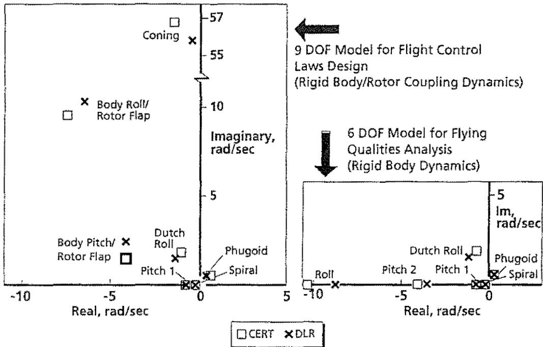
Figure 13. Comparison of poles from the 6 DOF and 9 DOF models identified by CERT and DLR
