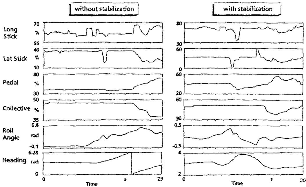
Figure 3. System identification control inputs for hover flight condition and roll and heading response. Flight tests without and with stabilization by the pilot
