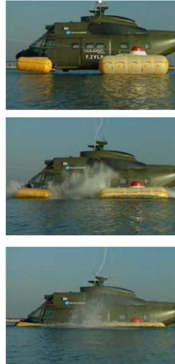
Fig. 22 – EC225 ditching tests – Full Scale
