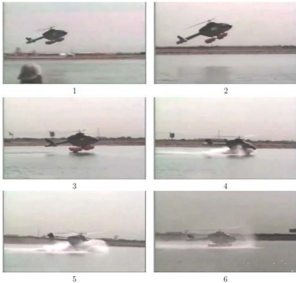
Fig. 3 – Typical helicopter water entry sequence in case of ditching (1 & 2 = Approach, 3 & 4 = Impact, 5 = Tranquilization, 6 = Stability, see [12])
