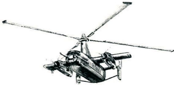
The Fairey Rotodyne 1957. 'Technology before its time'. Tip-jet drive, innovative and fast. The promise of the Rotodyne remains unfulfilled half a century later.
