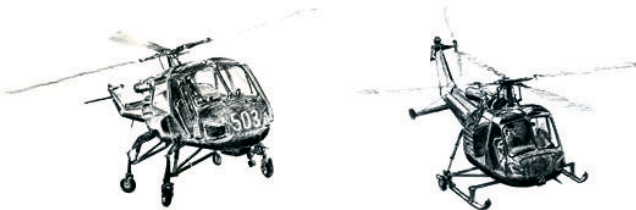
Both aircraft were derived from the Saunders-Roe P-531 1958 and the development was completed by Westland. The Scout, for the army in 1963, and the Wasp for small ship operations for the Royal Navy 1964.
