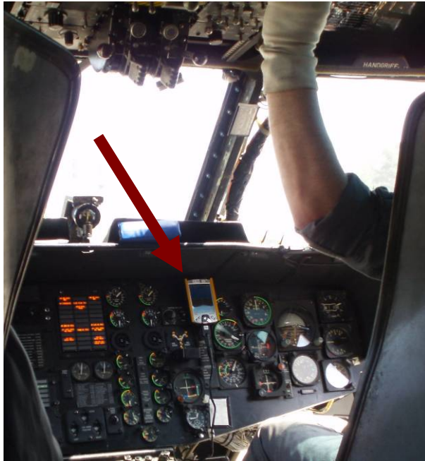
Figure 8: flight director display in CH53G cockpit
