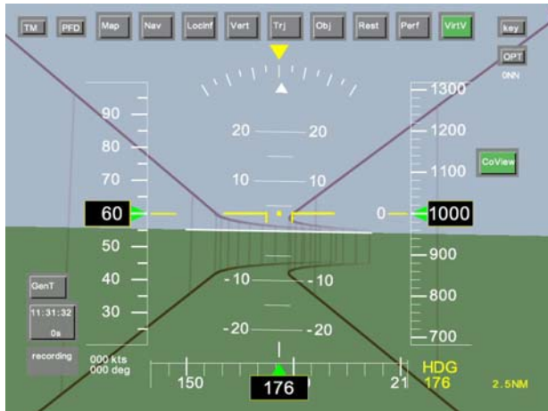
Figure 4: Enroute flight with tunnel display
