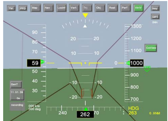
Figure 5: Approach flight with tunnel display
