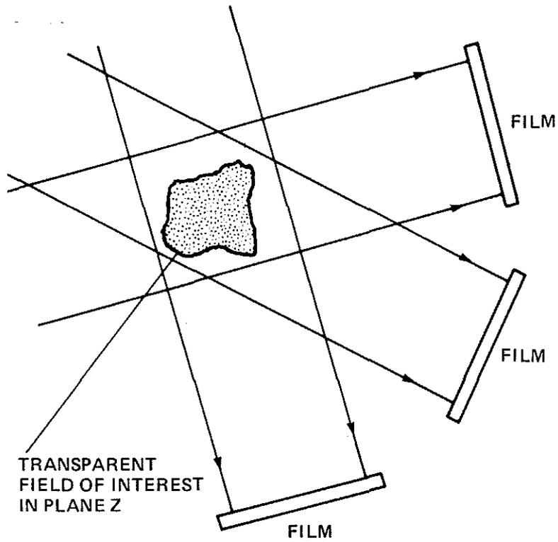
Fig. 7. Recording interferograms at various angles around the field of interest for tomographic reconstruction.
