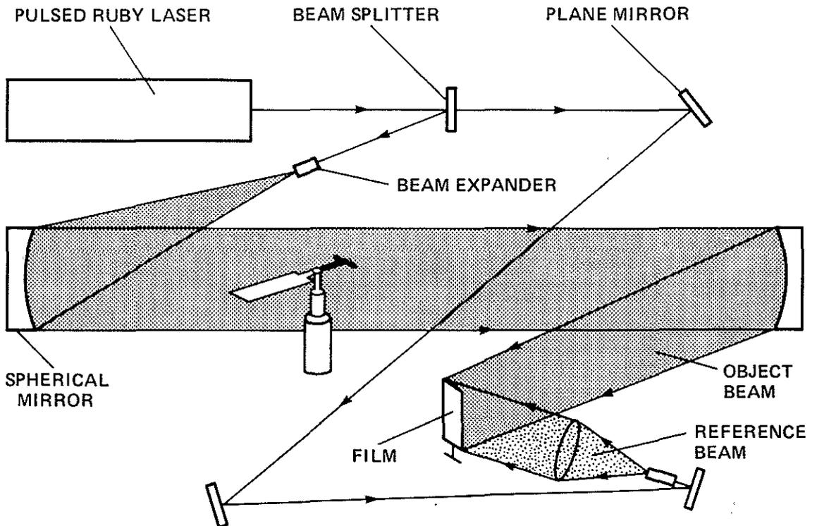
Fig. 8. Schematic drawing of the holographic recording system.
