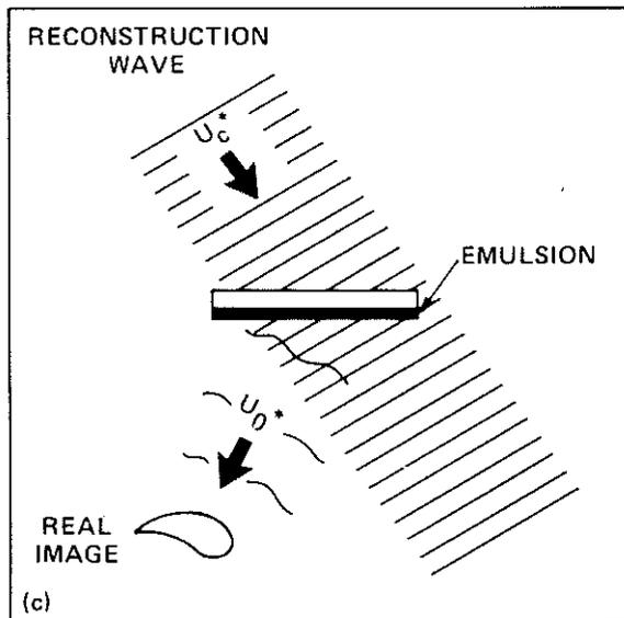
Physically, the first term in Eq. (2) represents the wave that is transmitted directly through the hologram. The second and third terms represent two first-order diffracted waves. The second, and most important, term of Eq. (2) can be written as  $(\beta U_R^* U_c) U_o$ , which is a replica of the original object wave. Thus, a virtual image of the original object has been reproduced.
