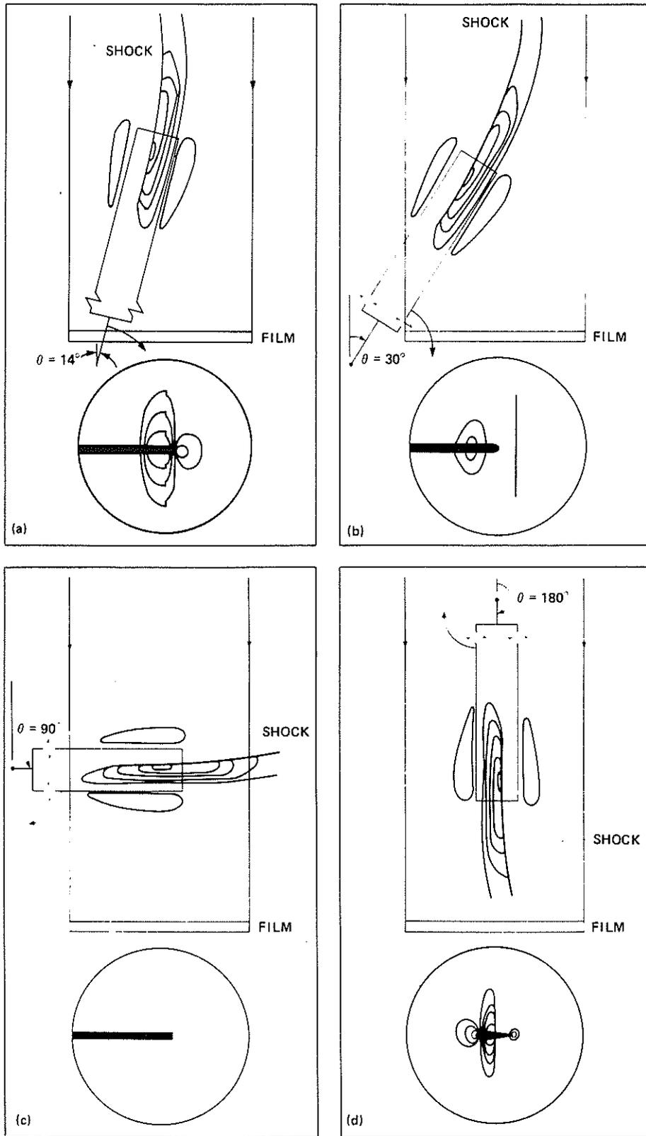
Fig. 10. Plan views of rotor blade with superimposed index of refraction contours, and expected appearance of interferograms at four different viewing angles. (a)  $\theta = 14^\circ$ . (b)  $\theta = 30^\circ$ . (c)  $\theta = 90^\circ$ . (d)  $\theta = 180^\circ$ .
