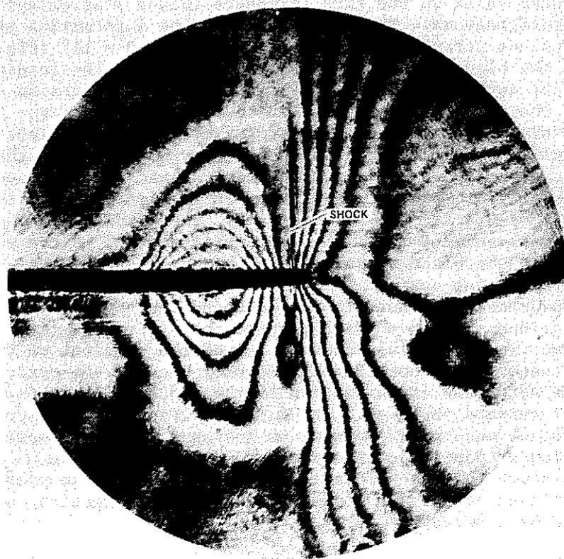
Fig. 12. Interferogram recorded at  $24^\circ$ .
