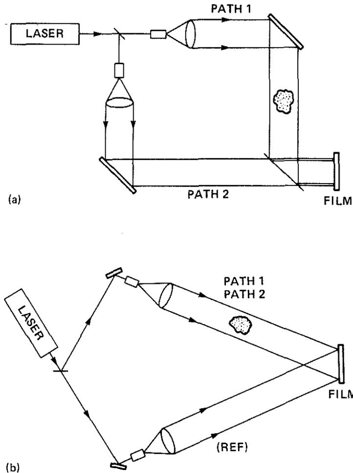
Fig. 5. Path differences of interfering waves. (a) Waves travel different paths at the same time in a Mach-Zehnder interferometer. (b) Waves travel the same path at two different times in a holographic interferometer. (Lower beam is reference wave.)
