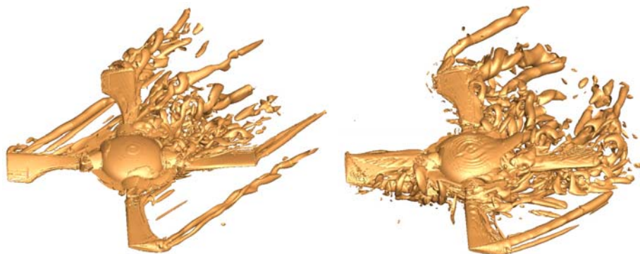
Figure 12 - Isosurface of Q criterion for steady (left) and unsteady (right) computations
