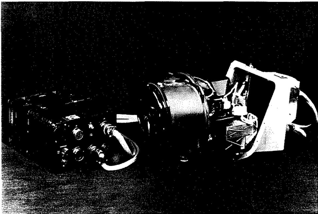
Fig. 4: CALIPSO FLIR, provided by TRT, with electronic box and serial-parallel scanning mechanism
