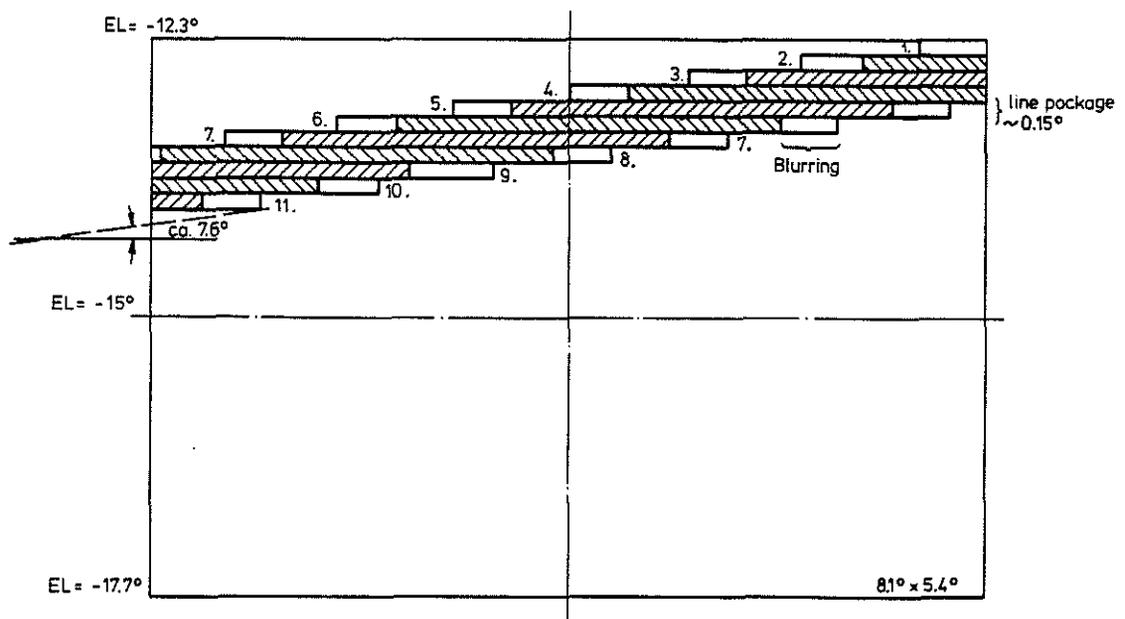
Fig. 9: Static video field with 100 % rotor speed. LOS is at El =  $-15^\circ$  in the LF. The serial-parallel FLIR scan mechanism cuts the rotor blade image into steps.
