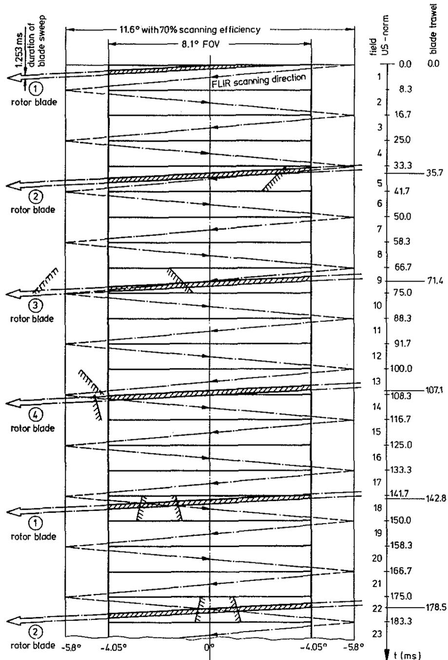
Fig. 19: Dynamic consideration of 23 separate US video fields with rotor blade influence for a mast-mounted CM FLIR with  $8.1^\circ \times 5.4^\circ$  FOV.
