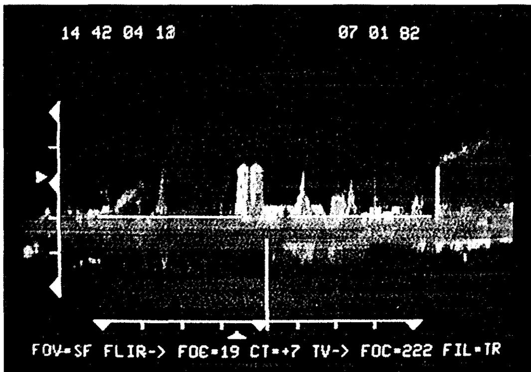
Fig. 7: Thermal image of the Munich Frauenkirche at a distance of 11.7 km taken with the CALIPSO FLIR
