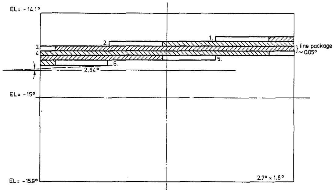
Fig. 12: Static video field at 100 % rotor speed. The LOS is at  $E_l = -15^\circ$  in the SF. The serial-parallel FLIR scan mechanism cuts the rotor blade image at this angle of elevation into approx. 2.4 steps, without blurring.
