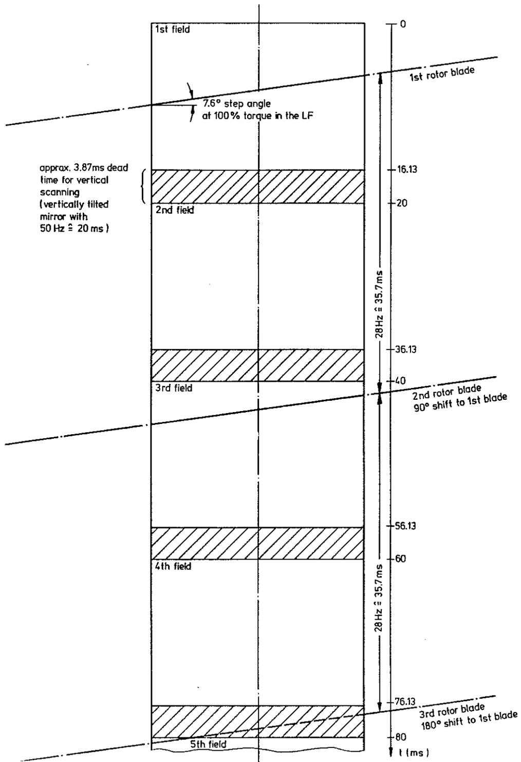
Fig. 14: Rotor blade influence on 5 separate video fields (100 ms) for the LF. (For explanation, see text).
