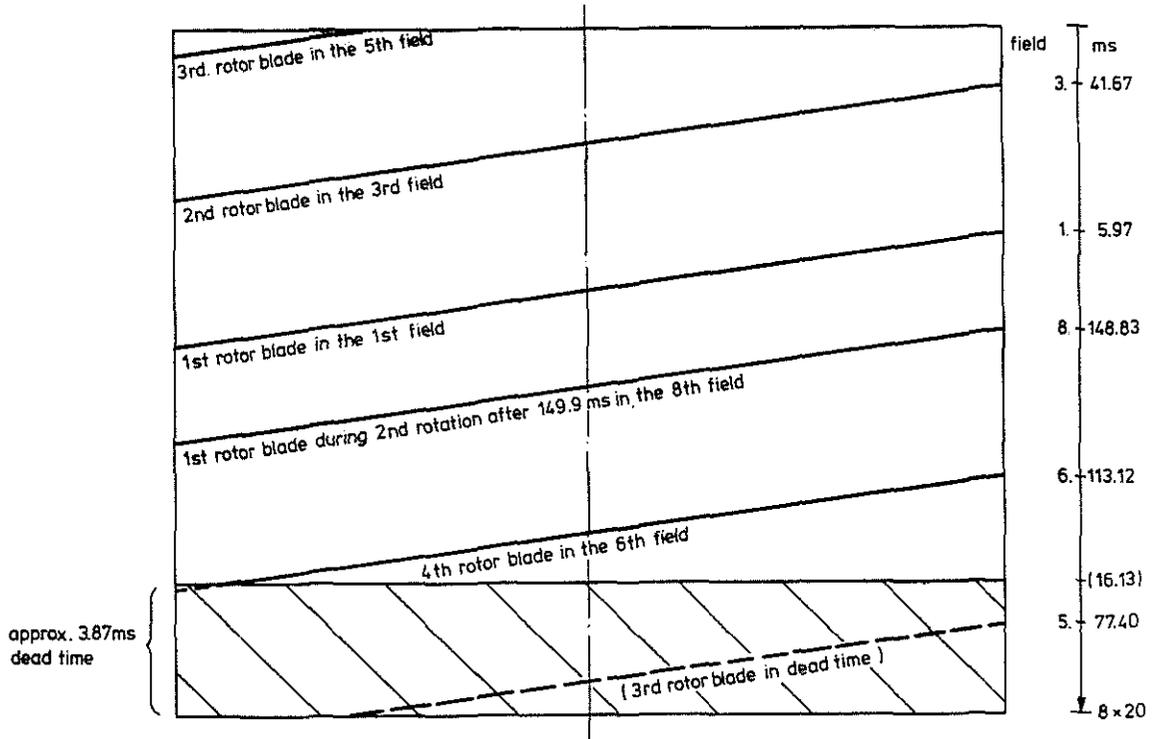
Fig. 15: Rotor blade influence demonstrated with 8 superimposed video fields (160 ms). In the dynamic case approx. 14 % of the LF image and 8 % of the SF image are vignettted in time, with only certain line packages, and not the whole image, being vignettted.
