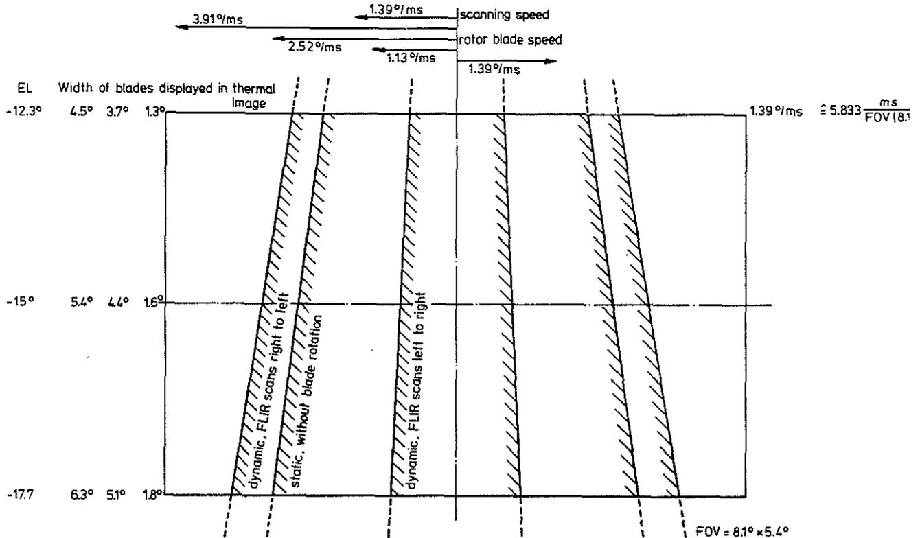
Fig. 18: Synthesis of static and dynamic cases for a rotor blade in the centre of an image taken with a CM FLIR for three superimposed stationary video fields.
